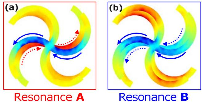
FIG. 4. (Color online) Current modes leading to a negative refractive index. The antisymmetric current mode (a) is excited by RCP at 4.7 GHz and the symmetric current mode (b) is excited by LCP at 6.2 GHz. The horizontal component of the excited currents is shown, where blue and red correspond to currents in opposite directions.
