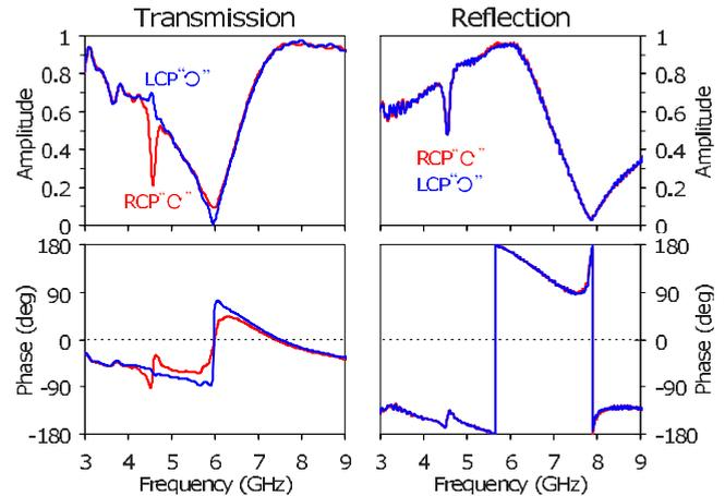
FIG. 7. (Color online) Amplitude and phase of the complex transmission and reflection coefficients  $T$  and  $R$  measured for the 3D-chiral bilayered metamaterial.
