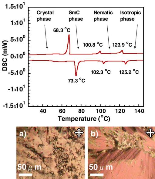
FIG. 2. (Color online) DSC chart of 8O-PBT-O4 obtained at a cooling rate of 10 °C/min and a heating rate of 10 °C/min, and texture images obtained using a polarized optical microscope at (a) 110 and (b) 90 °C.
