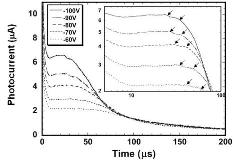
FIG. 5. Negative transient photocurrents in nematic phase measured at various applied voltages. The cell thickness was 4.8 µm. The arrows in the figure indicate transit times for fast and slow carriers.
