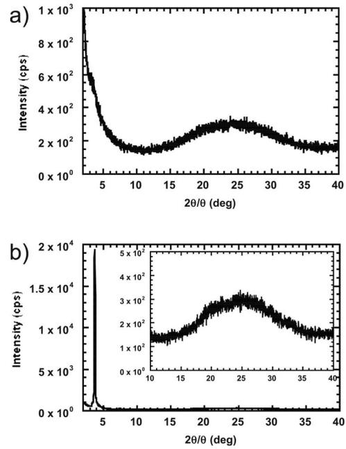
FIG. 3. XRD patterns of 8O-PBT-O4: (a) nematic phase at 110 °C and (b) smectic C phase at 90 °C.
