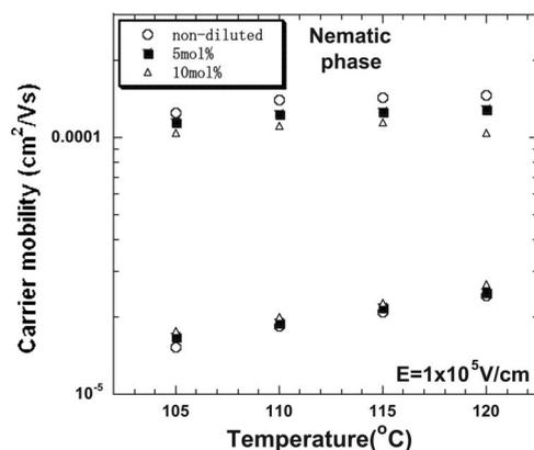
FIG. 7. Mobilities for positive carriers in nondiluted and diluted 8O-PBT-O4 containing 5 and 10 mol % *n*-tetradecane as a function temperature in the nematic phase. The cell thickness was 10  $\mu\text{m}$ .
