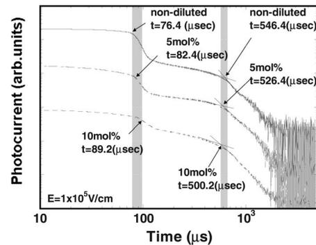
FIG. 6. Transient photocurrents for positive carriers in nondiluted and diluted 8O-PBT-O4 (moderately purified) containing 5 and 10 mol % *n*-tetradecane as a function of time in the nematic phase. The cell thickness was 10 µm.
