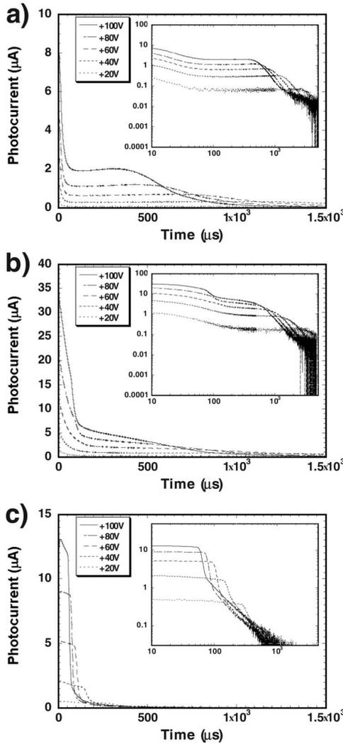
FIG. 4. Positive transient photocurrents measured by applying various voltages at 115 °C. The cell thickness was 10 µm. (a) Insufficiently purified 8O-PBT-O4, (b) moderately purified 8O-PBT-O4, and (c) highly purified 8O-PBT-O4.
