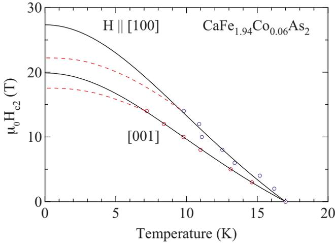
FIG. 3. (Color online) Temperature dependence of the upper critical field  $\mu_0 H_{c2}(T)$  of  $\text{CaFe}_{1.94}\text{Co}_{0.06}\text{As}_2$ . The dashed line is the value of  $\mu_0 H_{c2}$  estimated by WHH theory and the solid line is according to Ginzburg-Landau theory (see text for details).
