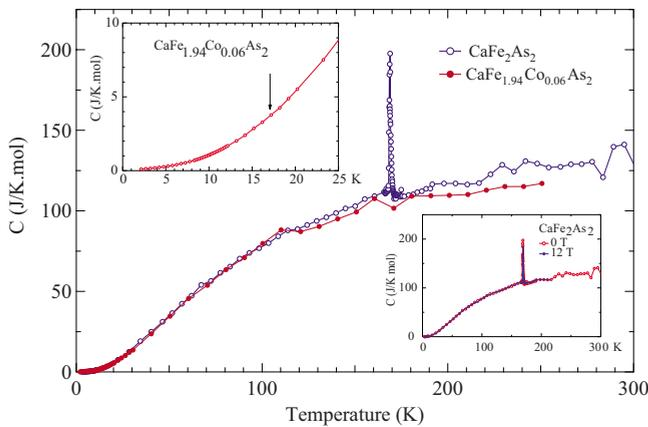
FIG. 4. (Color online) Temperature dependence of the heat capacity of  $\text{CaFe}_2\text{As}_2$  and  $\text{CaFe}_{1.94}\text{Co}_{0.06}\text{As}_2$ . The high-temperature SDW ordering is absent in the Co-doped sample. The lower inset shows the heat capacity of  $\text{CaFe}_2\text{As}_2$  in 0 and 12 T fields. The upper inset shows the temperature dependence of the heat capacity of  $\text{CaFe}_{1.94}\text{Co}_{0.06}\text{As}_2$  below 25 K.
