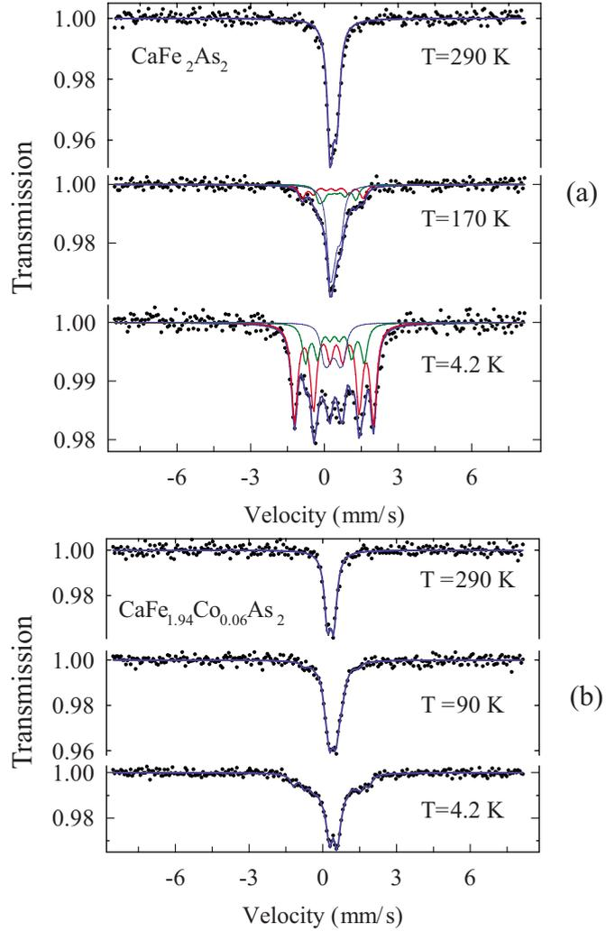
FIG. 5. (Color online) Mössbauer spectra of  $\text{CaFe}_2\text{As}_2$  and  $\text{CaFe}_{1.94}\text{Co}_{0.06}\text{As}_2$  at selected temperatures. For  $\text{CaFe}_2\text{As}_2$  the three subspectra at 4.2 K are shown (see text).
