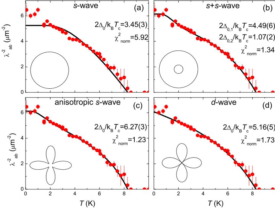
FIG. 3. (Color online) Temperature dependence of  $\lambda_{ab}^{-2}$  of FeSe<sub>0.85</sub> obtained from measured  $\sigma_{sc}$  by means of Eq. (3). The fitting curves (solid black lines) were obtained within the following models of the gap symmetries: (a) *s*-wave, (b) *s*+*s*-wave, (c) anisotropic *s*-wave, and (d) *d*-wave. The corresponding angular dependences of the gaps are shown as the insets.
