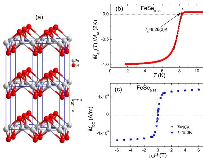
FIG. 1. (Color online) (a) The crystal structure of  $\alpha$ -FeSe. (b) Temperature dependence of the ac magnetization  $M_{ac}$  ( $\mu_0 H_{ac} = 0.1$  mT and  $\nu = 1000$  Hz) of FeSe<sub>0.85</sub>. (c) Dependence of dc magnetization  $M_{dc}$  on magnetic field at  $T = 10$  K and 150 K.
