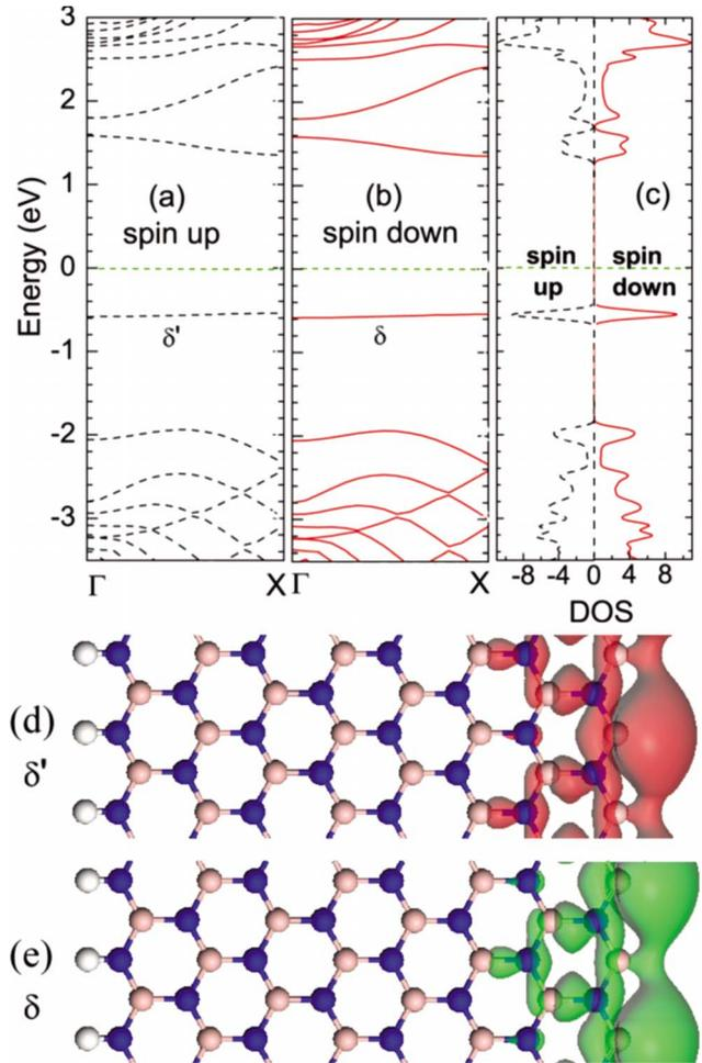
FIG. 4. (Color online) Electronic properties of 8-ZBNRR-HN. [(a)–(c)] Energy band structure. The  $\delta'$  and  $\delta$  bands are the highest valence bands. Energy zero is at the nominal Fermi-level position (i.e., the dash-dotted line). [(d)–(e)] Partial charge densities of the  $\delta'$  and  $\delta$  bands at the  $\Gamma$  point. The isosurface is  $0.03e/\text{Å}^3$ .
