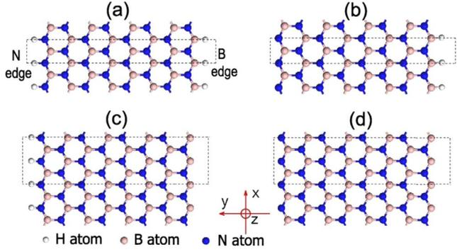
FIG. 1. (Color online) Atomic geometries of the relaxed ZBN-NRs with different edge treatments: (a) 8-ZBNNR-2H, (b) 8-ZBNNR-HB, (c) 8-ZBNNR-HN, and (d) pristine 8-ZBNNR, where the number 8 stands for the width of the ribbon, and the suffixes HB and HN stand for the hydrogen termination of the boron and nitrogen edges, respectively. The ribbons are infinitely long along the  $x$  direction. The dashed rectangles denote the unit cell of the systems.
