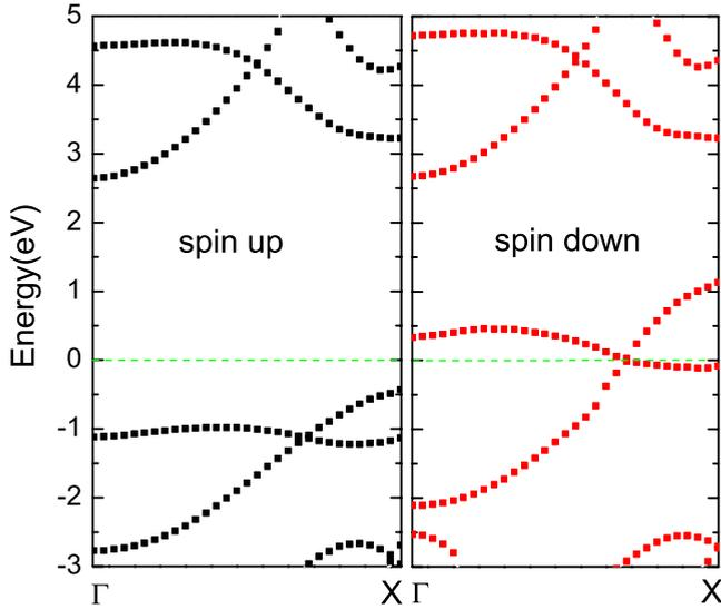
FIG. 3. (Color online) *GW* quasiparticle band structure for 3-ZBNRR-HB. Energy zero is at the Fermi level.
