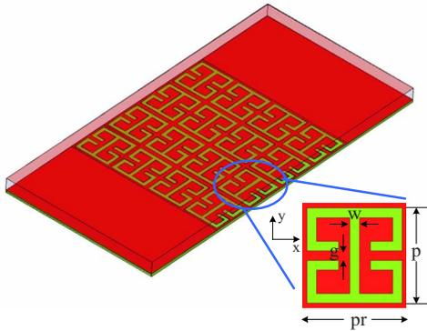
FIG. 2. (Color online) The CELC structure is chosen as the unit cell to realize the indefinite metamaterial.
