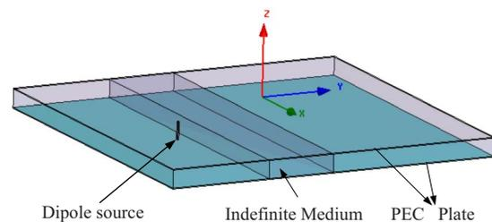
FIG. 1. (Color online) Theoretical model for partial focusing in a planar waveguide. An indefinite metamaterial slab is inserted into the waveguide, with a dipole source excitation.
