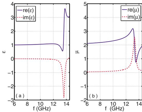
FIG. 5. (Color online) The effective permittivity and permeability curves for the simulation set up in Fig. 4(a). (a)  $\epsilon_z$ . (b)  $\mu_x$ .
