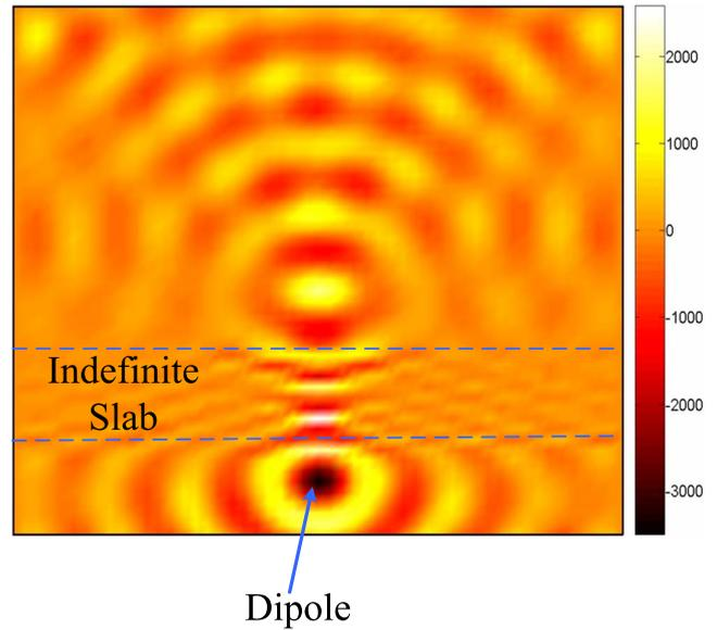
FIG. 7. (Color online) The distribution of simulated electric fields in a section of the planar waveguide at 11.5 GHz.
