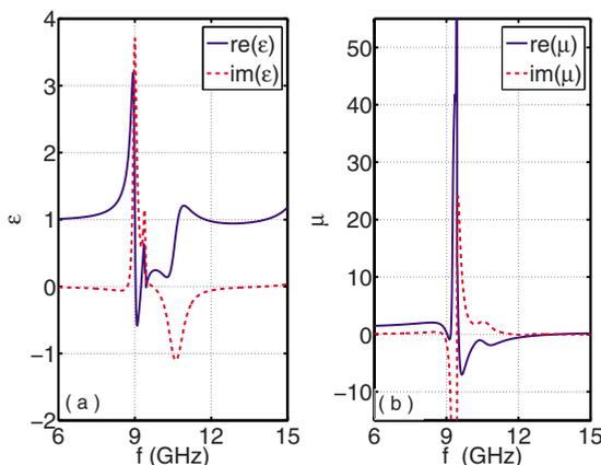
FIG. 6. (Color online) The effective permittivity and permeability curves for the simulation set up in Fig. 4(b). (a)  $\epsilon_z$ . (b)  $\mu_y$ .
