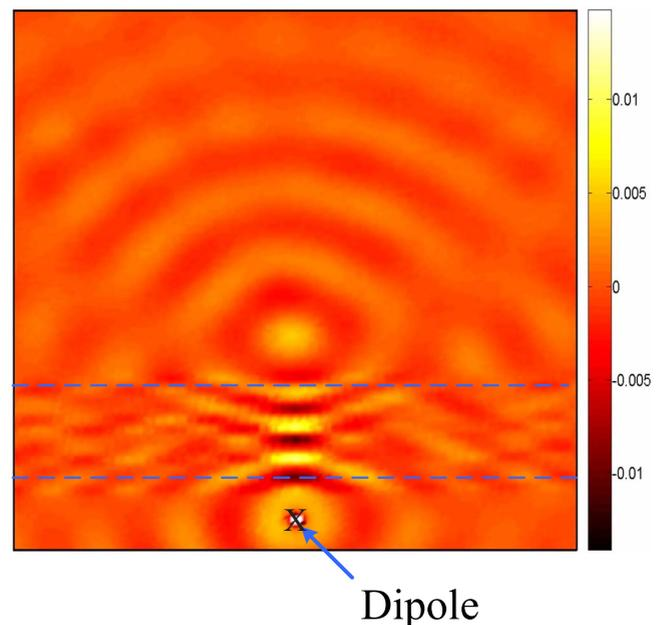
FIG. 8. (Color online) The experimental result for the electric field distributions inside the 2D mapper at 11.5 GHz.
