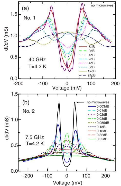
FIG. 1. (Color online) Differential conductance  $dI/dV$  for samples 1 and 2 as a function of the bias voltage  $V$  for the (a) 1- and (b) 5-k $\Omega$ -resistance break junctions at 4.2 K for different microwave power levels at (a) 40 and (b) 7.5 GHz.
