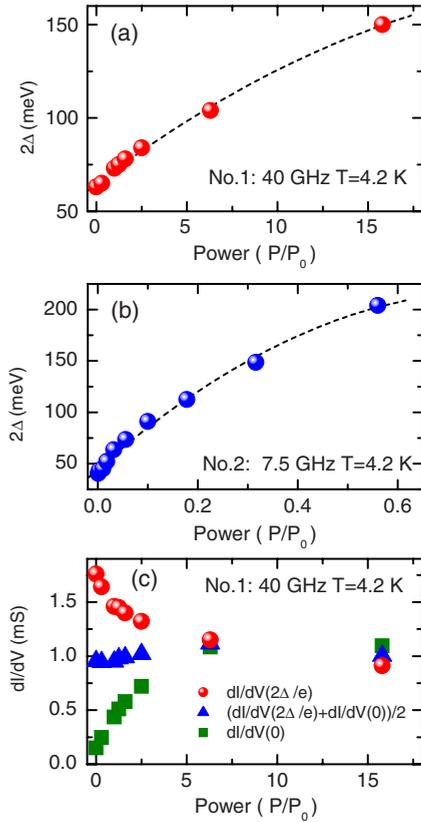
FIG. 2. (Color online) (a) and (b)  $2\Delta$  as a function of microwave power at  $T=4.2$  K for samples 1 and 2 at frequencies of 40 and 7.5 GHz, respectively. (c) Amplitudes of the gap maxima in  $dI/dV(V)$  curves at  $V=2\Delta/e$  and the magnitudes of the zero-bias conductance  $dI/dV$  as a function of 40-GHz microwave power for sample 1 extracted from Fig. 1(a).
