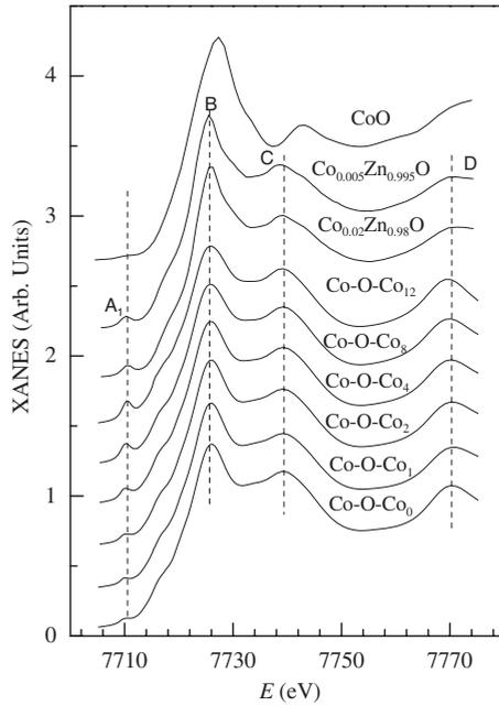
FIG. 2. Co  $K$ -edge XANES spectra of  $\text{Zn}_{1-x}\text{Co}_x\text{O}$  ( $x = 0.005, 0.02$ ) thin films, rock-salt structured CoO, and the calculated spectra for different structural models by replacing zero, one, two, four, eight, and twelve next-nearest Zn neighbors of  $\text{Co}_{\text{Zn}}$  with Co atoms.
