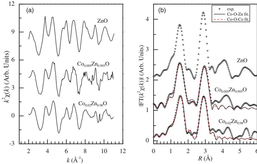
FIG. 1. (Color online) (a) Co  $K$ -edge EXAFS  $k^2\chi(k)$  functions for  $\text{Zn}_{1-x}\text{Co}_x\text{O}$  and the Zn  $K$ -edge function for ZnO powder, and (b) their Fourier transforms (empty circles). The solid lines and dashed lines in (b) show the fitting results by assuming all the next-nearest neighbors of Co to be Zn and Co, respectively. It is seen that in both cases, the fitting quality is almost equally good.
