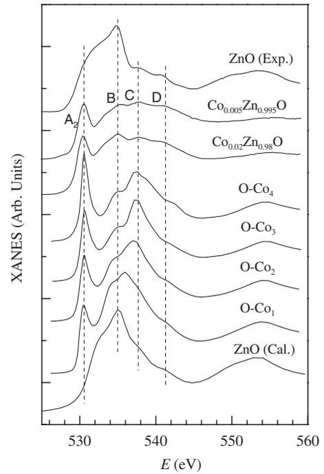
FIG. 3. O  $K$ -edge XANES spectra of  $\text{Zn}_{1-x}\text{Co}_x\text{O}$  ( $x = 0.005, 0.02$ ) thin films, ZnO powder, and the calculated spectra for different structure models by replacing one, two, three, and four Zn nearest neighbors of the absorbing O atom with Co.
