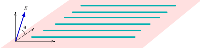
FIG. 1. (Color online) Array of one-dimensional chains formed by a two-dimensional optical lattice. The polarizing field E is directed perpendicular to the chains and at an angle \theta which can be used to tune the interchain interaction V_{\perp} in (2).
