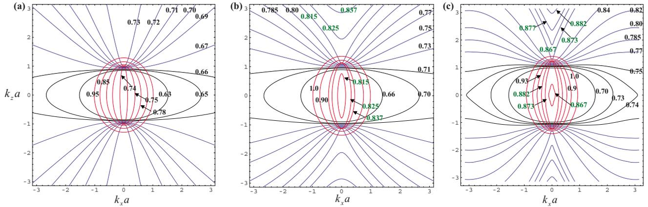
FIG. 4. (Color online) Isofrequency contours for an orthorhombic lattice of SRRs with the same parameters as in Fig. 2: (a) local model, (b) nonlocal model, and (c) full wave simulation. The insets indicate the value of the corresponding normalized frequency  $\omega a/c$ .
