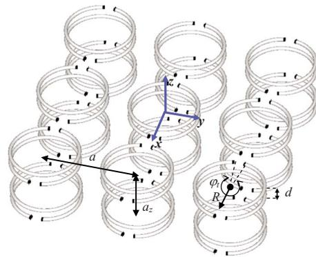
FIG. 1. (Color online) Geometry of an orthorhombic lattice  $a \times a \times a_z$  of broadside coupled SRRs. Each ring covers an angular sector defined by the angle  $\varphi$  and has mean radius  $R$ . The rings are made of metallic wires with radius  $r$ . The mean distance between rings is  $d$ .
