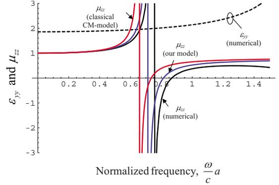
FIG. 2. (Color online) Effective permittivity and permeability of a lattice of SRRs with  $r_w = 0.005a$ ,  $d = 0.04a$ ,  $\varphi = 350^\circ$ ,  $R = 0.4a$ , and  $a_z = 0.5a$ .
