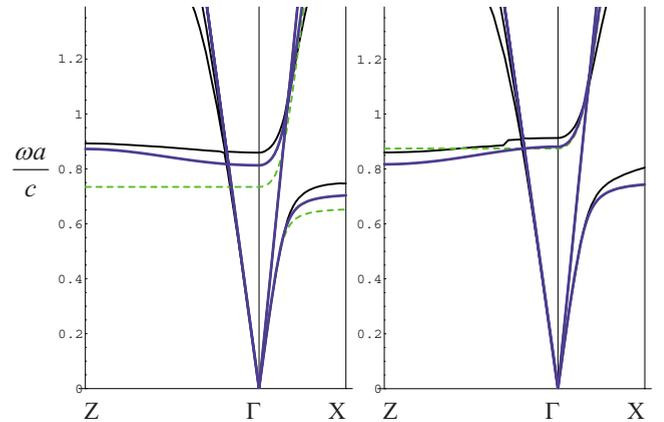
FIG. 3. (Color online) Left panel: Dispersion diagram for an orthorhombic lattice of SRRs. Right panel: Dispersion diagram for a bcc lattice of SRRs. The SRRs have the same parameters as in Fig. 2. Dashed (green/light gray) lines: CM-classical model. Solid (thick) blue/dark gray lines: nonlocal homogenization model. Solid (thin) black lines: full wave simulations.
