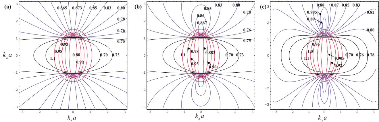
FIG. 5. (Color online) Isofrequency contours for a bcc lattice of SRRs: (a) local model, (b) nonlocal model, and (c) full wave simulation. The insets indicate the value of the corresponding normalized frequency  $\omega a/c$ .
