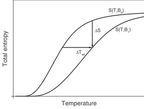
FIG. 1. Entropy vs temperature diagram illustrating the magnetoaloric potentials  $\Delta S$  and  $\Delta T_{ad}$ .
