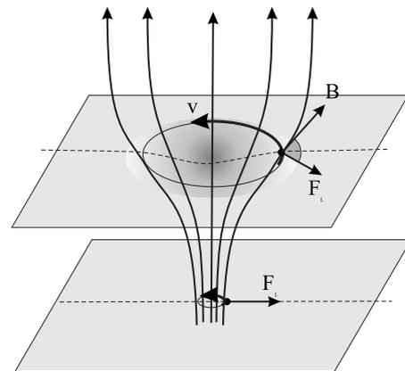
FIG. 1. Lorentz force acting on the circulating superconducting current. In the bulk, the Lorentz force is parallel to the surface. Near the surface, it is not parallel due to the magnetic stray field.
