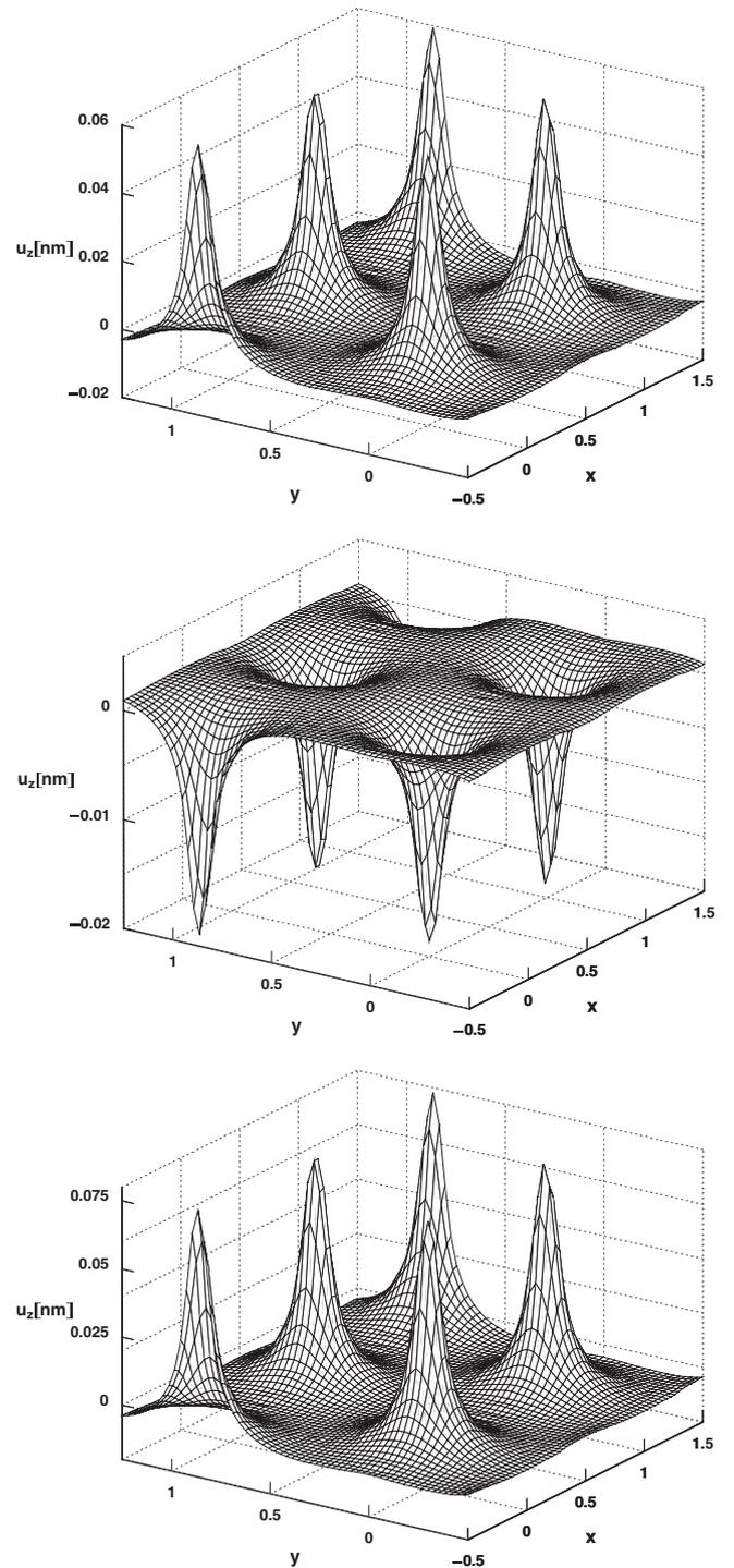
FIG. 3. Surface corrugation  $u_z(\mathbf{r})$  of  $\text{YBa}_2\text{Cu}_3\text{O}_7$  (top) as compared to the value neglecting surface dipoles (middle) and only surface dipoles (bottom). The temperature and the mean magnetic field are  $T=0.67$  and  $T_c=60$  K, and  $\bar{B}=0.01$  and  $B_{c2}(T)=0.6$  T. The length unit is the vortex distance  $a=58$  nm.
