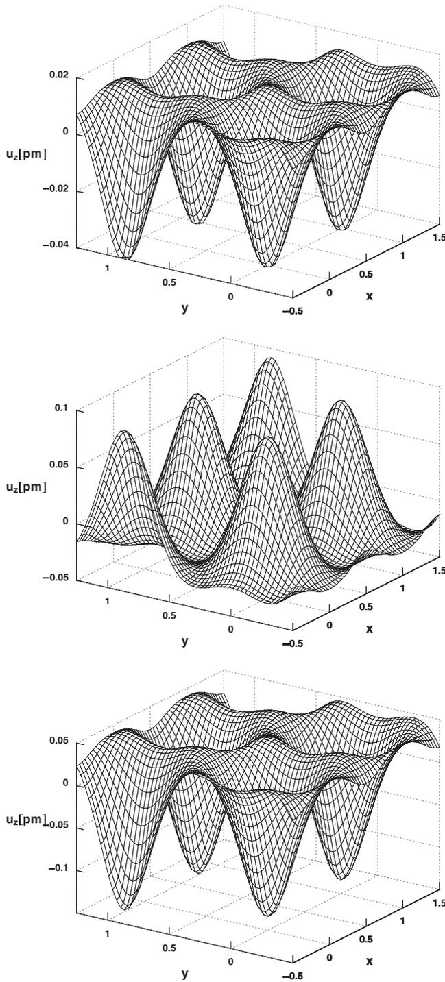
FIG. 2. Surface corrugation  $u_z(\mathbf{r})$  of Nb (top) compared to the value neglecting surface dipoles (middle) and only surface dipoles (bottom). The temperatures and the mean magnetic fields are  $T=0.95$  and  $T_c=9$  K, and  $\bar{B}=0.21$  and  $B_{c2}(T)=6.4$  mT. The length unit is the vortex distance  $a=128$  nm.
