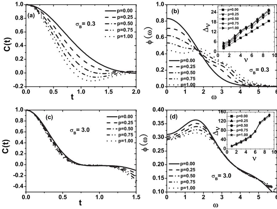
FIG. 1. Time-dependent correlation functions and the corresponding spectral densities for the two typical cases. The system undergoes a crossover from a central-peak behavior to a collective-mode behavior when  $\sigma_J=0.3$ ; however, when  $\sigma_J=3.0$ , the crossover vanishes and the system only shows a behavior between a central-peak behavior and a collective-mode one. The insets of (b) and (d) present the recurrent  $\Delta_\nu(\nu=1, \dots, 9)$ .
