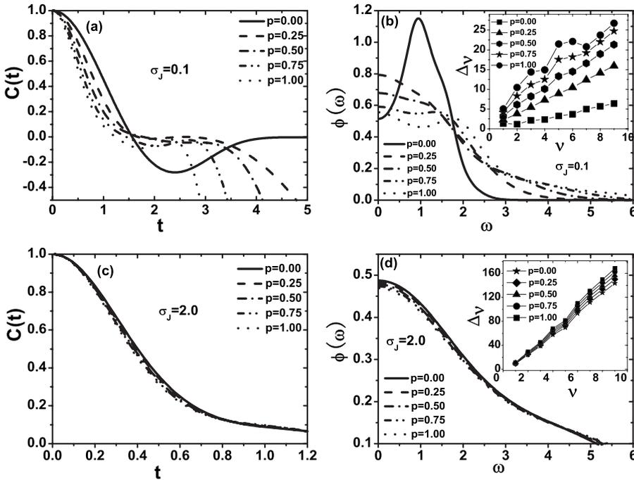
FIG. 2. Autocorrelation functions and spectral densities for the case that the bonds satisfy the double-Gaussian distribution, while  $B=1$ . The standard deviations take two typical values  $\sigma_J = 0.1$  and  $2.0$ . By comparing the insets of (b) and (d), we can conclude that the recurrants fall on a straight line as  $\sigma_J$  increases.
