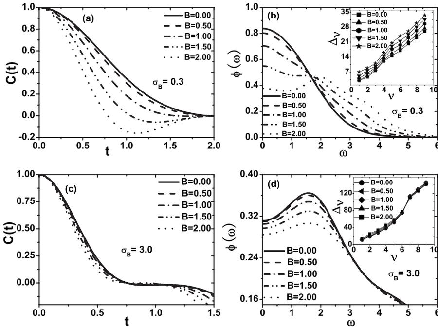
FIG. 4. Autocorrelation functions and the corresponding spectral densities for two groups of different parameters when the random fields satisfy Gaussian distribution. When the standard deviation is small ( $\sigma_B=0.3$ ), (a) and (b) show that the dynamics of the system changes from a central-peak behavior to a collective-mode one as the mean value of  $B_i$  increases from 0 to 2; however, when  $\sigma_B=3.0$ , the system is only in a most disordered state.
