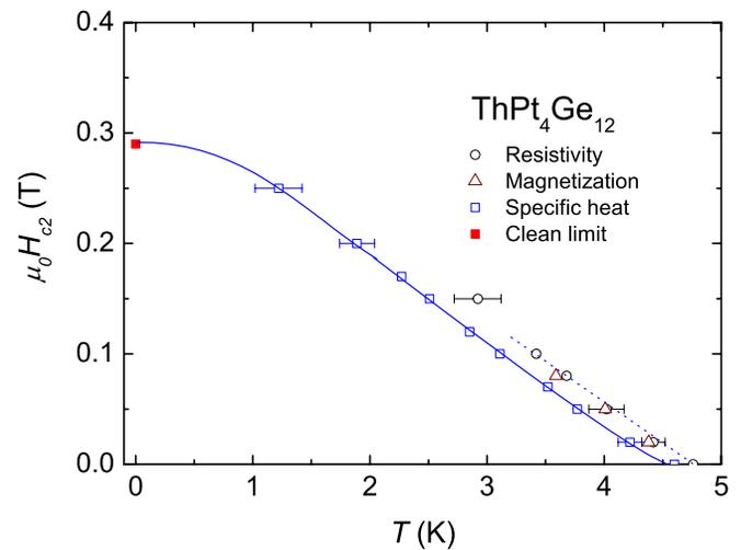
FIG. 4. (Color online) Upper critical field versus temperature determined for  $\text{ThPt}_4\text{Ge}_{12}$  from the resistivity (circles), magnetization (triangles), and specific heat (squares) data. Filled square represents the calculated value of  $H_{c2}(0)$  in the clean limit. Solid line emphasizes a linear variation of  $H_{c2}$  with temperature.
