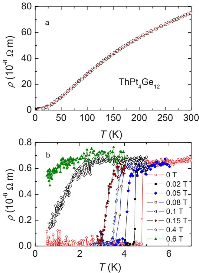
FIG. 1. (Color online) (a) Temperature dependence of the electrical resistivity of  $\text{ThPt}_4\text{Ge}_{12}$ . For the sake of clarity, only every 15th experimental point is displayed. The solid line is the WC fit described in the text. (b) Low-temperature resistivity measured in zero and several nonzero applied magnetic fields.
