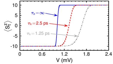
FIG. 2. (Color online) The effect of intrinsic relaxation processes on magnetic switching of the molecule  $Mn_{12}$  in the limit of high LUMO level, calculated for indicated values of the relaxation time,  $\tau_R$ , and for parallel magnetic configuration. The polarization parameters of the electrodes are  $P_L = 1$  and  $P_R = 0.5$ . The other parameters are  $J_\lambda = 100$  meV,  $D \approx 0.05$  meV (Ref. 14),  $T = 0.01$  K, and  $c = 10$  kV/s.
