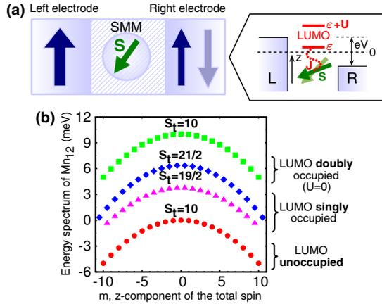
FIG. 1. (Color online) (a) Schematic representation of the system and switching mechanism due to spin-polarized current. (b) Energy levels of the  $Mn_{12}$  molecule for the following parameters:  $D \approx 0.05$  mV,  $D_1 \approx -0.006$  meV,  $D_2 \approx 0.0017$  meV (Ref. 14),  $J = 0.25$  meV,  $\varepsilon = 5$  meV, and  $U = 0$ . Different parabolas correspond to indicated values of the SMM's total spin  $S_t$  and occupation numbers of the LUMO level.
