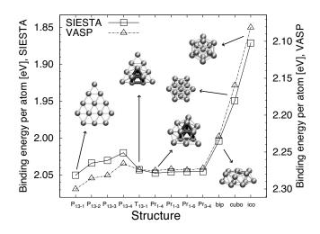
FIG. 8. Comparison of the binding energies per atom (in eV) in different cluster structures obtained with LCAO (SIESTA) and planewave (VASP) basis functions. The left (SIESTA) and right (VASP) energy axes have been vertically shifted so that the results for the  $T_{13-1}$  cluster overlap.
