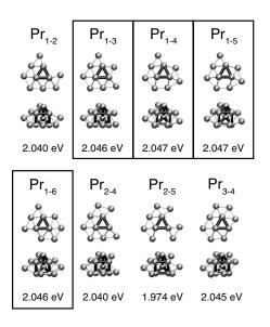
FIG. 6. Structures and binding energies per atom for the eight prism clusters (top and side views). The trigonal prism is highlighted. The framed structures were found by scanning the potential-energy surface using the MD/CG procedure described in Sec. II, while the remaining structures were constructed from the 15-atom parent cluster. See text for details.
