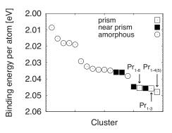
FIG. 5. Binding energies per atom for a series of cluster structures obtained through the procedure outlined in the text. The values for the icosahedral (1.87 eV) and cuboctahedral (1.95 eV)  $Au_{13}$ clusters are outside the displayed range. Three groups can be distinguished: amorphous (left), near prism (center), and prism (right).
