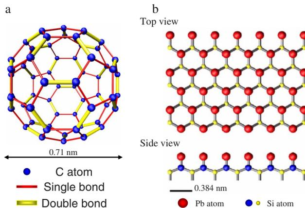
FIG. 1. (Color online) Atomic model of the C<sub>60</sub> molecule (a) and of the Pb/Si(111)-(1 × 1) structure (b).
