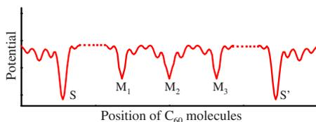
FIG. 6. (Color online) Schematic potential diagram for the diffusion of a  $C_{60}$  molecule at the Pb-covered surface. The horizontal axis is the one-dimensional representation of the position of the molecule at the surface.  $S$  and  $S'$  represent stable adsorption states and  $M_i$  represents a metastable adsorption state.
