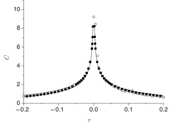
FIG. 4. Three-state Potts model. MC data (open circles) and SE data (small solid boxes) for specific heat. The continuous line represents the specific heat calculated from Eqs. (44) and (45).
