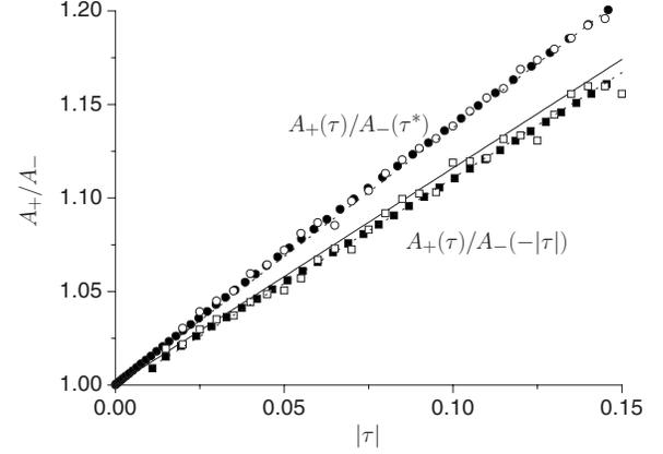
FIG. 3. The effective-amplitude ratio  $A_+(\tau)/A_-(-|\tau|)$  at symmetric reduced temperatures. The SE data are indicated by closed circles and the MC data by open circles. The ratio  $A_+(\tau)/A_-(\tau^*)$  at dual reduced temperatures is denoted by closed squares in the case of the SE data and by open squares for the MC data. The upper dashed line is the prediction equation (40).
