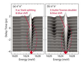
FIG. 3. (Color online) Differential reflectivity spectra as a function of the delay time for (a)  $\sigma^+\sigma^+$  and (b)  $\sigma^+\sigma^-$  pump and probe. The  $\sigma^+$  pump (vertical arrow) is tuned to the exciton resonance (1625.7 meV).
