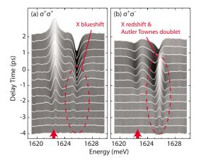
FIG. 4. (Color online) Differential reflectivity spectra as a function of the delay time for (a)  $\sigma^+\sigma^+$  and (b)  $\sigma^+\sigma^-$  pump and probe. The  $\sigma^+$  pump (vertical arrow) is tuned close to the biexciton resonance (1621.8 meV).
