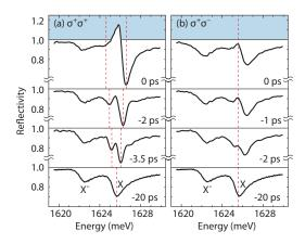
FIG. 2. (Color online) Reflectivity spectra collected at various delay times for a  $\sigma^+$  pump tuned to the exciton resonance (1625.7 meV). The vertical scale is the same for all spectra. (a)  $\sigma^+$  probe, the dashed lines indicate the position of the Stark split modes. (b)  $\sigma^+$  probe, the dashed-line indicates the position of the pump pulse.
