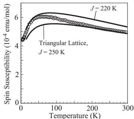
FIG. 2. Temperature dependence of the spin susceptibility of randomly oriented samples of  $\text{EtMe}_3\text{Sb}[\text{Pd}(\text{dmit})_2]_2$ . Solid curves show the result of the [7/7] Padé approximants for the high-temperature expansion of the regular-triangular antiferromagnetic spin- $1/2$  system with  $J=220$  and 250 K.
