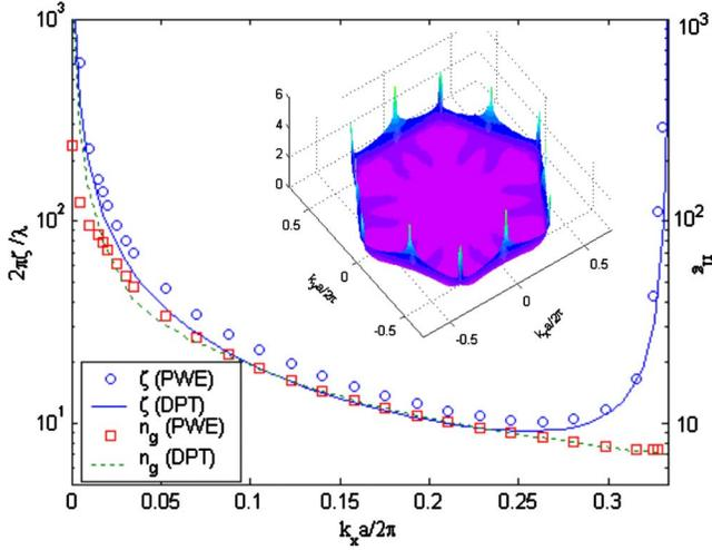
FIG. 2. (Color online) The dispersion surface curvature and group index on the MK line for the lower branch of the first band. The inset plots  $\log_{10}\left(\frac{2\pi|\zeta|}{\lambda} + 1\right)$  in the 1 BZ for this branch.
