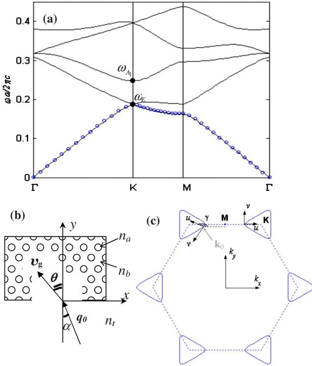
FIG. 1. (Color online) A triangular lattice. (a) Photonic bands for a structure:  $n_a=3.8$ ,  $n_b=1.33$ ; and  $r=0.3a$ ; lines: PWE method; circles: DPT method. The two lowest bands have IRREPs  $E$  and  $A_1$  at  $K$ . (b) Schematic of a typical experimental configuration. (c) A typical dispersion surface for the lower branch of the first band.
