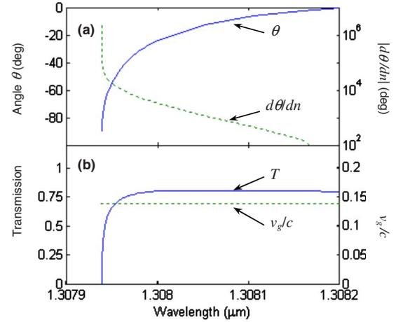
FIG. 4. (Color online) Normalized transmission and sensitivities for modes near the degenerate  $\omega_E$  mode of the first band,  $\omega_E a/2\pi c \sim 0.187$ ,  $\alpha = 27.9^\circ$ ,  $n_1 = n_a$ .
