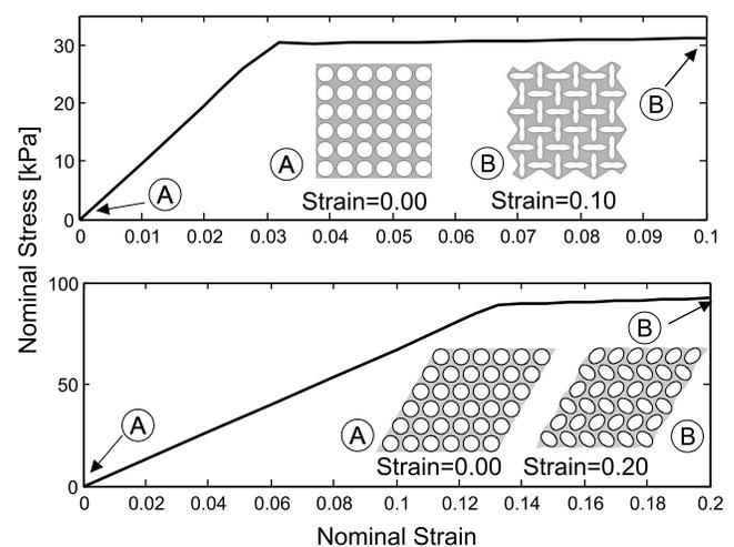
FIG. 1. Nominal stress vs nominal strain curves during axial compression in the vertical direction for the square (top) and hexagonal (bottom) arrays of circular holes. The departure from linearity is the result of an elastic buckling in the microstructure that triggers a pattern transformation.
