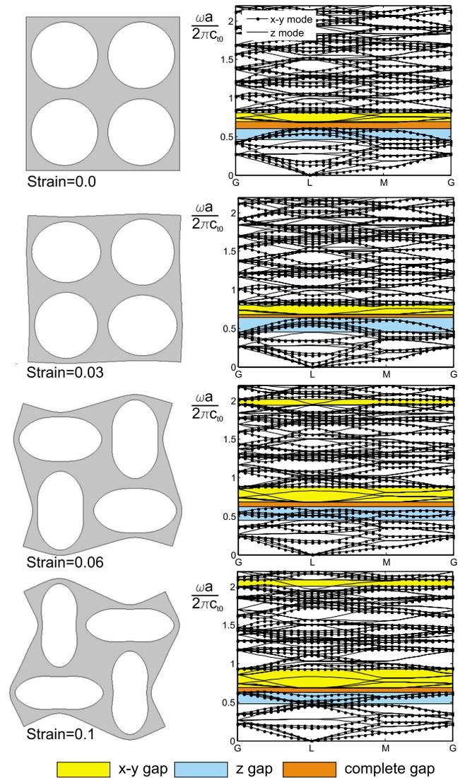
FIG. 3. (Color online) Phononic band gap structure for the square array of circular holes with  $r=4.335$  mm and  $a_x=a_y=9.97$  mm ( $f_0=0.59$ ) at different levels of macroscopic nominal strain in the elastomer matrix ( $c_{t0}=32.2$  m/s). In-plane (labeled  $x$ - $y$ ) and out-of-plane (labeled  $z$ ) modes are reported together with the  $x$ - $y$ ,  $z$ , and complete band gaps. The points  $G$ ,  $L$ , and  $M$  are defined in Fig. 2.
