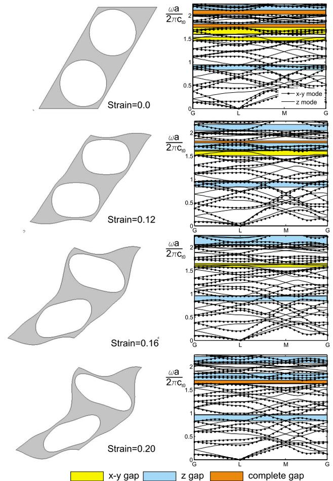
FIG. 5. (Color online) Phononic band gap structure for the oblique array of circular holes with  $r=4.335$  mm,  $a_x=10.97$  mm, and  $a_y=9.47$  mm ( $f_0=0.57$ ) at different levels of macroscopic nominal strain in the elastomer matrix ( $c_{t0}=32.2$  m/s). In-plane (labeled  $x$ - $y$ ) and out-of-plane (labeled  $z$ ) modes are reported together with the  $x$ - $y$ ,  $z$ , and complete band gaps. The points  $G$ ,  $L$ , and  $M$  are defined in Fig. 2.
