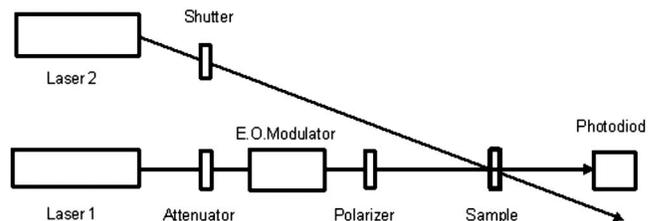
FIG. 1. Experimental installation.
