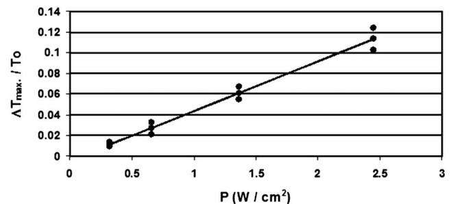
FIG. 5. Relative transparency changes vs pump beam intensity.
