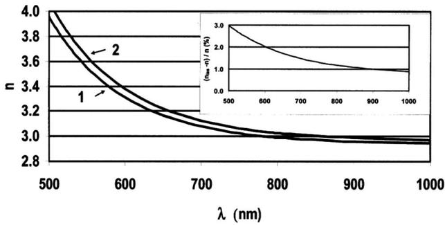
FIG. 6. Refractive index spectra for nonirradiated film and film under irradiation. Inset: relative change of refractive index under irradiation.
