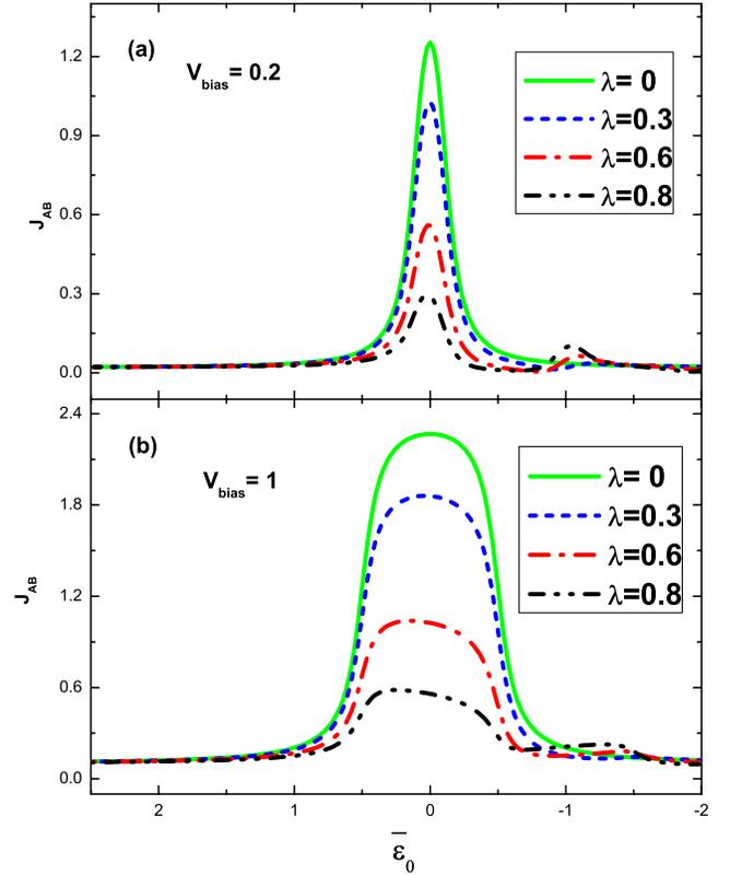
FIG. 4. (Color online) Current  $J_{AB}$  vs the renormalized level  $\bar{\epsilon}_0$  for different  $e$ -ph interaction strengths  $\lambda$  with  $\Gamma=0.1$ ,  $\phi=0$ , and  $t_{\text{ref}}=0.1$ .
