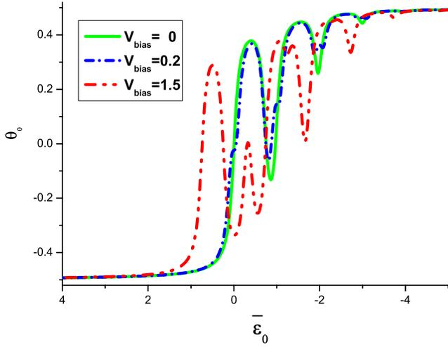
FIG. 6. (Color online) Phase  $\theta_0$  vs the level  $\bar{\epsilon}_0$  for the different bias  $V_{\text{bias}}$ . The other parameters are  $\lambda=0.6$ ,  $\Gamma=0.1$ , and  $t_{\text{ref}}=0.1$ .
