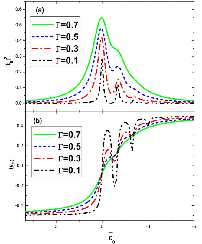
FIG. 2. (Color online) Transmission probability  $|t_0|^2$  (a) and transmission phase  $\theta$  (b) vs the renormalized level  $\bar{\epsilon}_0$  for different  $\Gamma$  with the  $e$ -ph interaction strength  $\lambda=0.7$ .
