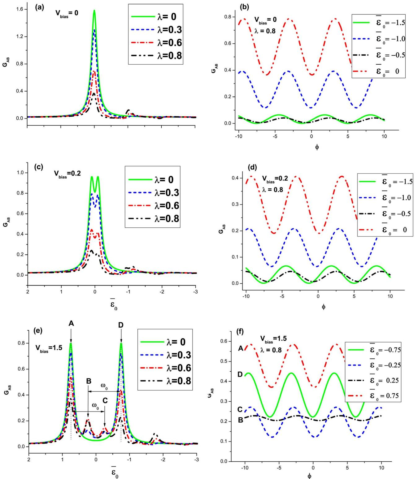
FIG. 5. (Color online) (a),(c),(e) Differential conductance  $G_{AB}$  vs the level  $\bar{\epsilon}_0$  for the bias  $V_{\text{bias}}=0$  (a), 0.2 (c), and 1.5 (e) at  $\phi=0$ . (b),(d),(f) Differential conductance  $G_{AB}$  vs the magnetic flux  $\phi$  for the bias  $V_{\text{bias}}=0$  (b), 0.2 (d), and 1.5 (f). The other parameters are  $\Gamma = 0.1$  and  $t_{\text{ref}}=0.1$ .
