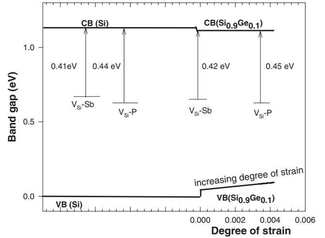
FIG. 3. Schematic representation illustrating the variation of the valence band and conduction band of  $\text{Si}_{0.9}\text{Ge}_{0.1}$  with respect to that of Si as well as the  $E$  center energy level as a function of degree of strain. For clarity, the horizontal scale is applied only for  $\text{Si}_{0.9}\text{Ge}_{0.1}$ .
