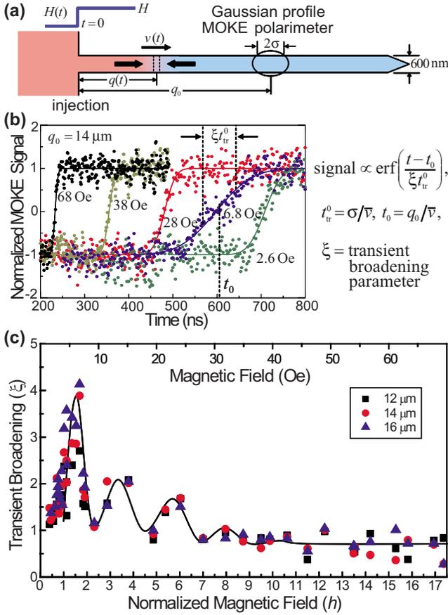
FIG. 2. (Color online) (a) Schematic of DW velocity measurement. (b) Measured transients at different values of  $H$ , showing transient broadening effect characterized by the parameter  $\xi$ . (c) Plot of  $\xi(h)$  for several values of  $q_0$ .
