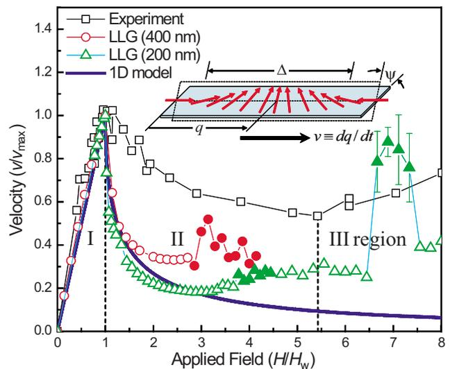
FIG. 1. (Color online) Measured and simulated DW velocity [normalized to  $v_{\max} \equiv v(H_W)$ ] as a function of applied field (normalized to the Walker field  $H_W$ ). Walker breakdown occurs at  $H = H_W$  corresponding to  $\psi = \pi/4$ . (Inset) Schematic description of the spin distribution within a propagating transverse DW showing tilt angle  $\psi$  and wall width  $\Delta$ . Solid symbols for LLG simulations designate onset of noise in simulated velocity described later in text.
