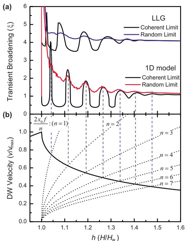
FIG. 4. (Color online) (a) Transient broadening parameters versus reduced field obtained from 1D model and LLG simulations (for 200 nm width) in coherent and incoherent limits. In the simulations,  $2\sigma=2\ \mu\text{m}$  and  $q_0=8.5\ \mu\text{m}$  were used. The LLG results are vertically offset for clarity. (b) Intersection of the function of the  $2x_0f/n$  with the mobility curve (normalized parameters) showing condition for maximum broadening.
