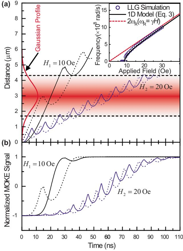
FIG. 3. (Color online) (a) Numerical simulations of DW displacements in a 20 nm thick  $\times$  200 nm wide permalloy nanowire versus time for two values of  $H$  above  $H_w$ . Gaussian profile centered around  $q_0 = 3 \mu\text{m}$  represents MOKE beam. (Inset) DW frequency determined by numerical simulations. (b) Simulated MOKE signal produced by the four displacement records.
