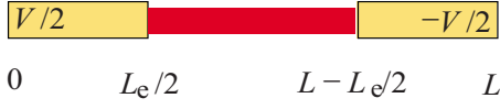
FIG. 1. (Color online) One-dimensional model for an insulator, to which two metallic electrodes are attached.
