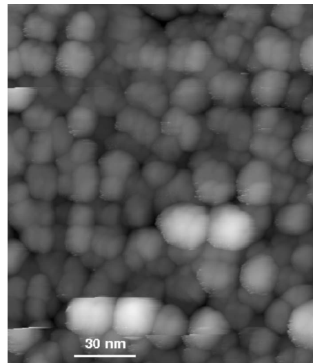
FIG. 1. A typical atomic force microscopy photograph (reproduced from Ref. 11) of Pb grains deposited on the insulating \text{SiO}_2 plate. Each grain is individually superconducting with its own phase. The mean size of the grain is of the order of 20 nm, while the intergrain distance is 1 order smaller, i.e., is about 2 nm.
