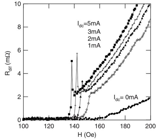
FIG. 3. Differential resistance as a function of field with various bias dc currents at 70.0 K. Amplitude of the applied ac current is 1 mA. With increasing bias current, the fields of the steps or the peaks, which are signs of the vortex-lattice melting transition, are suppressed.
