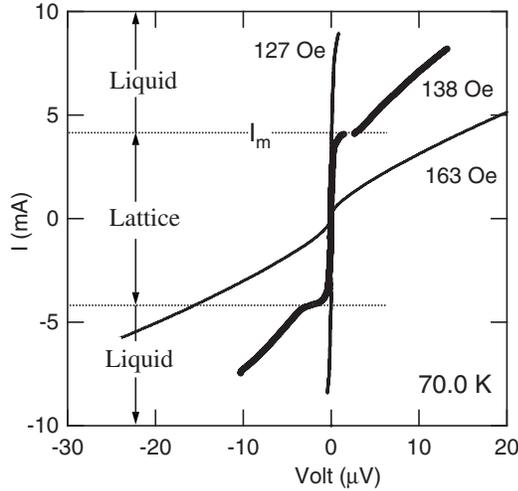
FIG. 4.  $I$ - $V$  characteristic in 138 Oe which shows a melting transition induced by the  $c$ -axis current (a bold line). Sharp jumps in the voltage are observed at  $I_m$ .  $I_m$  increases with decreasing magnetic fields. As comparisons,  $I$ - $V$  curves in higher and lower fields are plotted by thinner lines.
