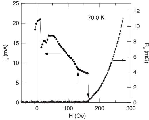
FIG. 2. Magnetic field dependence of the  $c$ -axis critical current and the  $c$ -axis resistance at 70 K are plotted in the left and right axes, respectively. Anomalies corresponding to the melting transition of vortex lattice are observed by both measurements in different fields: 131 Oe for  $I_c$  and 163 Oe for  $R_c$ .
