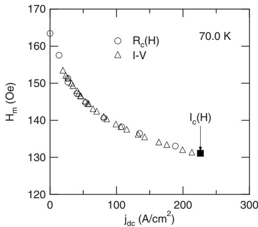
FIG. 5. Bias current dependence of the fields of the melting transition at 70 K. Circles and triangles are data from  $R(H)$  and  $I$ - $V$  measurements, respectively. A point obtained from  $I_c(H)$  as the melting transition is added by a solid square.  $H_m$  decreases monotonically, as the bias current increases.
