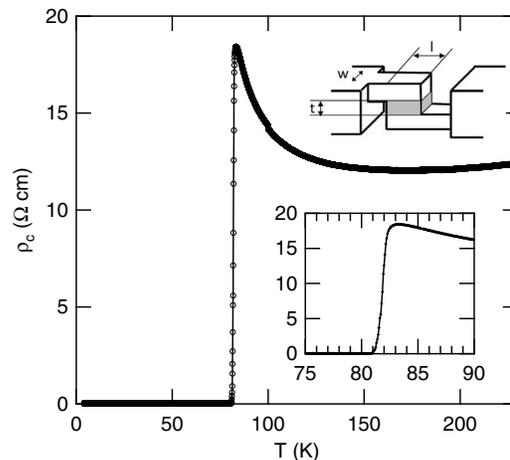
FIG. 1. Temperature dependence of the  $c$ -axis resistivity. A part near the superconducting transition is magnified in the lower inset. The upper inset shows a schematic draw of the sample shape.
