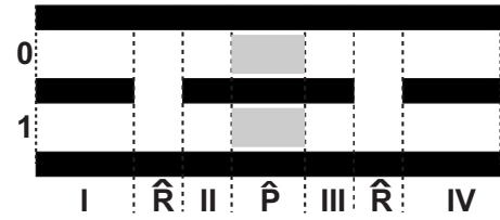
FIG. 6. Schematic representation of the Mach-Zehnder interferometer. We have indicated the three quantum-operation regions, consisting of the two coupling windows \hat{R} and one phase gate \hat{P} , and four other segments where the qubit state is well defined (see Table I).
