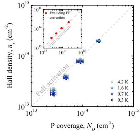
FIG. 2. (Color online) Comparison of the measured Hall densities  $n_s$  at different measurement temperatures. For clarity, only data at four temperatures are presented. Inset: Corresponding classical Hall densities (solid circles) obtained after eliminating the EEI correction from the respective Hall coefficients (note that both axes are defined in the same way as for the main graph). The dashed lines represent full electrical activation.
