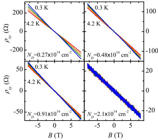
FIG. 1. (Color online) Plots of the Hall resistivity  $\rho_{xy}$  as a function of perpendicular magnetic field  $B$  for Si:P  $\delta$ -doped samples at temperatures of 0.3, 0.7, 1.6, and 4.2 K (only four temperatures are shown here for clarity).
