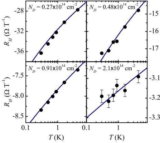
FIG. 3. (Color online) Semilogarithmic plots of the measured Hall coefficient  $R_H$  vs temperature  $T$  for Si:P  $\delta$ -doped samples with different doping densities. Lines are fits to the data using electron-electron interaction theory [Eq. (3)] described in the text.
