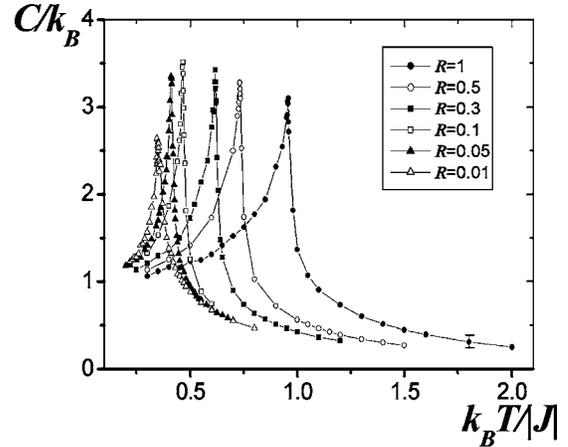
FIG. 3. Dependence of the heat capacity  $C/k_B$  on temperature  $k_B T/|J|$  for system with  $L=24$ .
