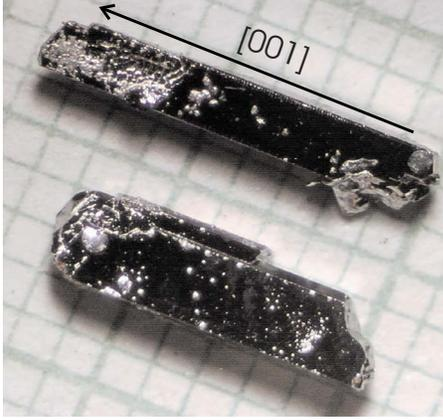
FIG. 1. (Color online) As grown  $\text{GdMn}_{2.21(4)}\text{Al}_{9.79(4)}$  crystal on a millimeter scale paper, depicting typical dimensions of the  $\text{RMn}_{2+x}\text{Al}_{10-x}$  crystals and the crystallographic direction.
