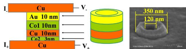
FIG. 1. (Color online) Schematic structure and SEM image for the vertical stack of Co rings.
