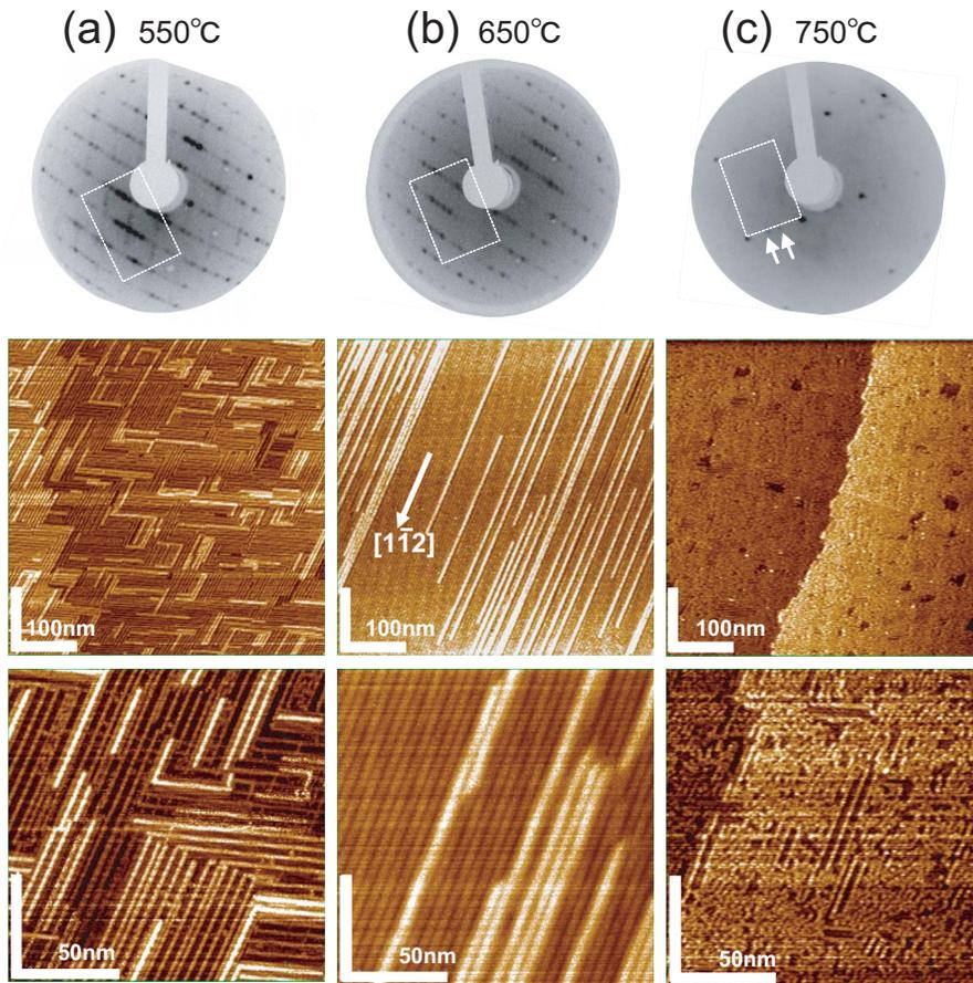
FIG. 2. (Color online) LEED and STM images of the surfaces after 30 min annealing at (a) 550 °C, (b) 650 °C, and (c) 750 °C, with the dc along  $[1\bar{1}2]$ . LEED patterns are recorded at incident beam energy of 65 eV. STM image is obtained in constant-current mode with sample bias voltage of 1 V. Sizes of STM images are  $500 \times 500 \text{ nm}^2$  (top) and  $150 \times 150 \text{ nm}^2$  (bottom).
