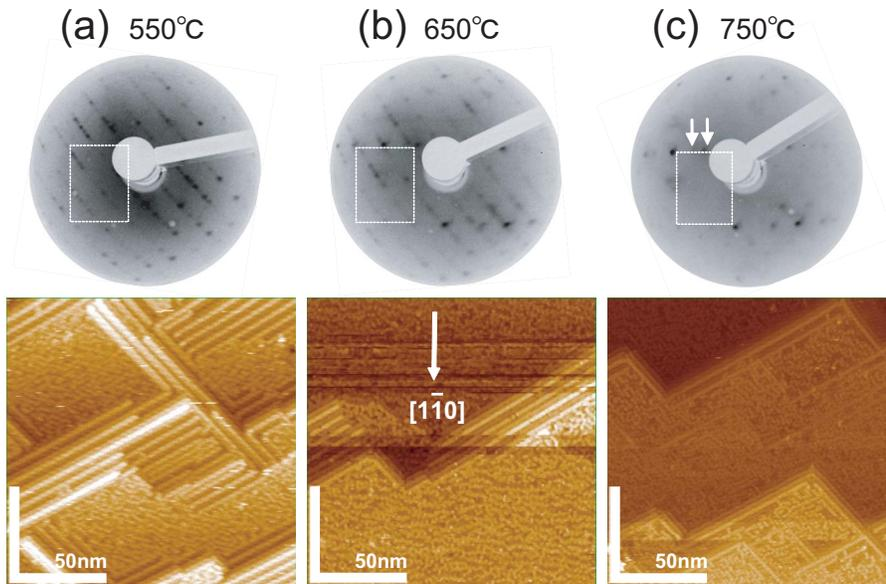
FIG. 3. (Color online) LEED and STM images of the surfaces after 30 min annealing at (a) 550 °C, (b) 650 °C, and (c) 750 °C, with the dc along  $[1\bar{1}0]$ . LEED patterns are recorded at incident beam energy of 65 eV. STM image is obtained in constant-current mode with sample bias voltage of 1 V. Size of STM image is  $150 \times 150 \text{ nm}^2$ .
