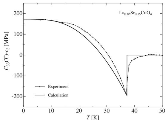
FIG. 12. Comparison between the theoretical and experimental temperature dependences of the elastic constant  $C_{33}(T) - c_3$  in  $\text{La}_{0.85}\text{Sr}_{0.15}\text{CuO}_4$ . The experimental data were taken from Ref. 14. For the parameter values used, see the text.
