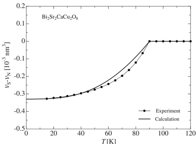
FIG. 11. Comparison between the theoretical and experimental temperature dependences of the volume change  $v_S - v_N$  in  $\text{Bi}_2\text{Sr}_2\text{CaCu}_2\text{O}_8$ . The experimental data were taken from Ref. 13. For the parameter values used, see the text.
