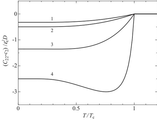
FIG. 6. Temperature dependence of the elastic constant  $C_{22}(T)$  for different values of  $g_2/g_1$  in the  $s$ -wave SC state. The same parameter values of  $g_1 D$  and  $\epsilon_c/k_B$  as in Fig. 1,  $\zeta_2=1.0$  and  $\eta_1=1.0$  have been assumed. The lines 1, 2, 3, and 4 have been calculated for  $g_2/g_1=-1.9, -1.0, 1.0,$  and  $1.9$ , respectively.
