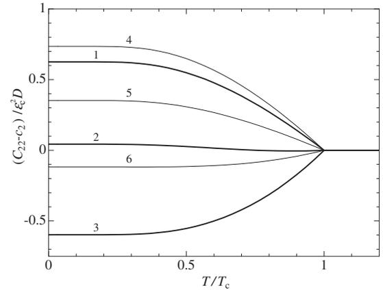
FIG. 5. Temperature dependence of the elastic constant  $C_{22}(T)$  in the  $s$ -wave SC state. The same parameter values of  $g_1 D$  and  $\epsilon_c/k_B$  as in Fig. 1, and  $g_2/g_1 = -1.9$  have been assumed. The bold lines 1, 2, and 3 have been calculated for  $\eta_1 = 1.5, 0.5,$  and  $-0.5,$  respectively, under common  $\zeta_2 = -2.5.$  The thin lines 4, 5, and 6 have been calculated for  $\zeta_2 = -2, -1,$  and  $0,$  respectively, under common  $\eta_1 = 2.$
