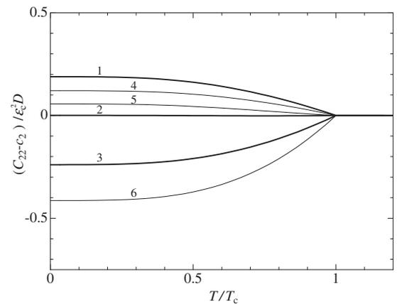
FIG. 9. Temperature dependence of the elastic constant  $C_{22}(T)$  in the  $d_{x^2-y^2}$ -wave SC state. The same parameter values of  $g_2 D$  and  $\epsilon_c/k_B$  as in Fig. 2, and  $g_1/g_2 = -0.47$  have been assumed. The bold lines 1, 2, and 3 have been calculated for  $\eta_2 = 2.5, 2,$  and  $1.5$ , respectively, under common  $\zeta_2 = -2.5$ . The thin lines 4, 5, and 6 have been calculated for  $\zeta_2 = -2, -1,$  and  $0$ , respectively, under common  $\eta_2 = 2$ .
