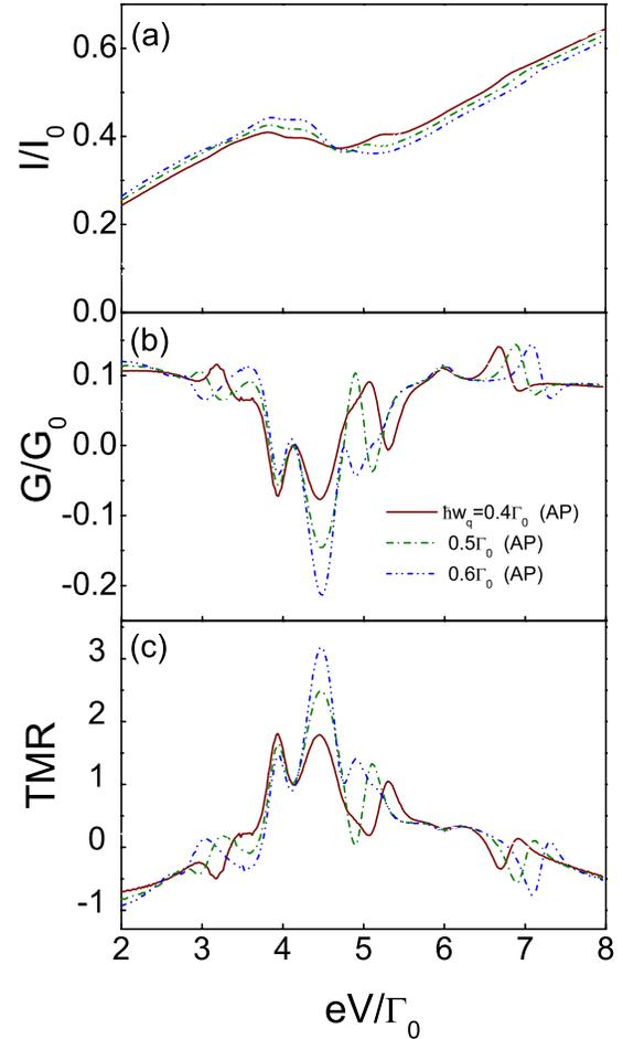
FIG. 3. (Color online) Bias dependence of (a) the tunnel current  $I$ , (b) the differential conductance  $G$ , and (c) TMR for the different  $\hbar\omega_q$ , where  $\gamma=0.2$ ,  $\varepsilon_{\uparrow}=3.0\Gamma_0$ , and  $\varepsilon_{\downarrow}=2.0\Gamma_0$ .
