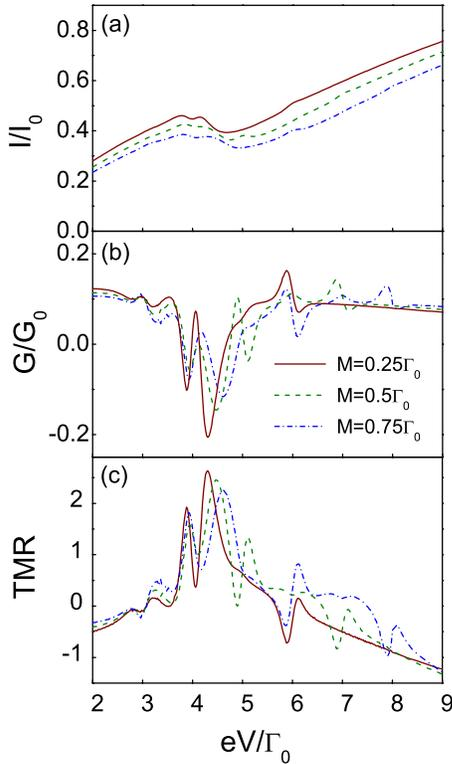
FIG. 6. (Color online) Bias dependence of (a) the tunnel current  $I$ , (b) the differential conductance  $G$ , and (c) TMR for different molecular fields of the middle FM layer, where  $\gamma=0.2$ ,  $\varepsilon=2.5\Gamma_0$ , and  $\hbar\omega_q=0.5\Gamma_0$ .
