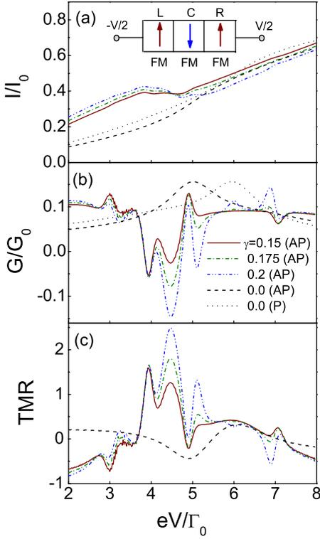
FIG. 1. (Color online) Bias dependence of (a) the tunnel current  $I$ , (b) the differential conductance  $G$ , and (c) TMR for the different  $\gamma$ , where  $\hbar\omega_q = 0.5\Gamma_0$ ,  $\varepsilon_{\uparrow} = 3.0\Gamma_0$ , and  $\varepsilon_{\downarrow} = 2.0\Gamma_0$ .
