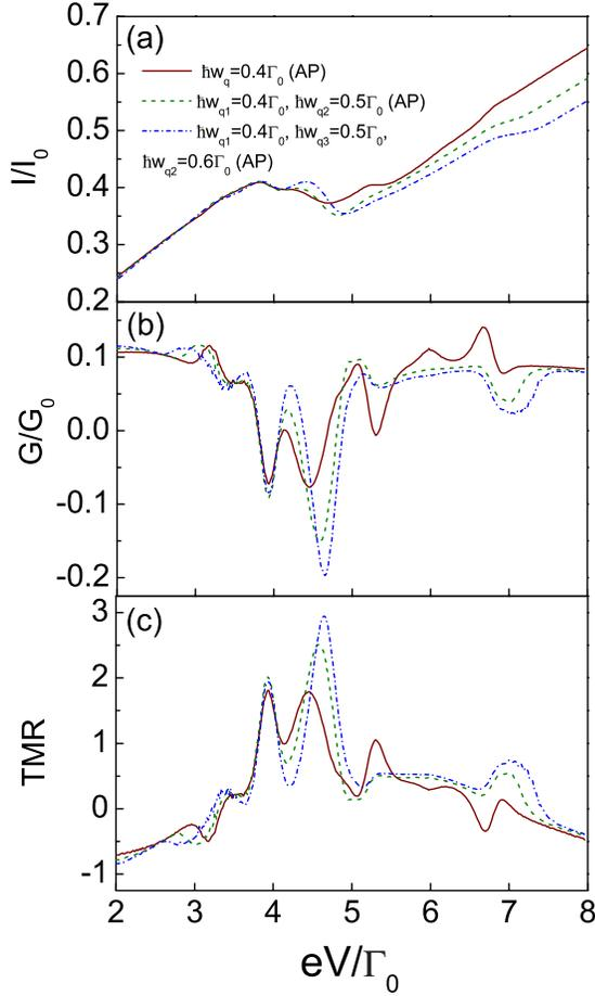
FIG. 4. (Color online) Bias dependence of (a) the tunnel current  $I$ , (b) the differential conductance  $G$ , and (c) TMR for different spin-wave modes, where  $\gamma=0.2$ ,  $\varepsilon_{\uparrow}=3.0\Gamma_0$ , and  $\varepsilon_{\downarrow}=2.0\Gamma_0$ .
