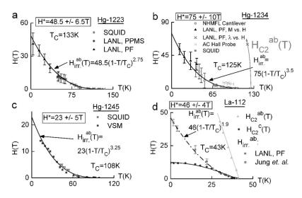
FIG. 2. Determination of  $H^*$  using various magnetic measurements of  $H^{ab}_{irr}(T)$ : (a) Hg-1223, (b) Hg-1234, (c) Hg-1245, and (d) La-112. In (b) and (d) dashed lines indicate  $H^{ab}_{c2}(T)$  from TDO measurements. In (d) we also illustrate  $H^c_{c2}$  for comparison. We note reasonable consistency among different experimental techniques, indicating strong suppression of  $H^* \equiv H^{ab}_{irr}(0)$  relative to  $H^{ab}_{c2}(0)$  (or  $H_p$ ) in all cuprates.
