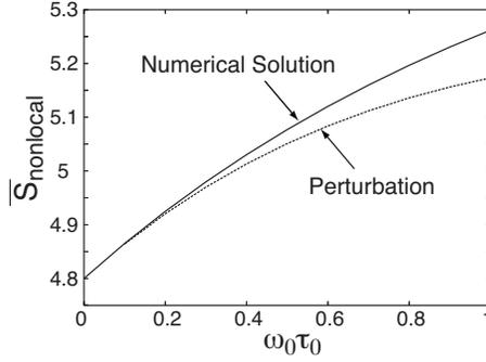
FIG. 8. The normalized bounce action  $\bar{S}$  as a function of the cutoff parameter  $\tau_0$  obtained by numerical calculation (solid line) and perturbative method (dotted line). In the limit  $\omega_0\tau_0 \rightarrow 0$ , the bounce action becomes 4.8, which corresponds to the local approximation.
