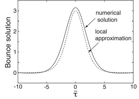
FIG. 7. Numerically obtained bounce solution for the action with the Ohmic nonlocal  $\beta$  term for  $\omega_0\tau_0=1$  is shown by the solid line. The usual bounce solution for the action with local approximation, which is given by  $\psi_0(\tilde{\tau})=3/\cosh^2(\tilde{\tau}/2)$ , is also shown by the broken line.
