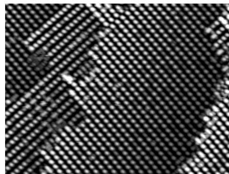
FIG. 7. 525 \times 390 \text{ \AA}^2 filled-state STM image of the \text{In}/\text{Si}(100)4 \times 3 magic cluster array which is almost completely (by \sim 93\% ) built of Pb-modified clusters. The array was prepared by saturating Pb adsorption at 330 \text{ }^\circ\text{C} .
