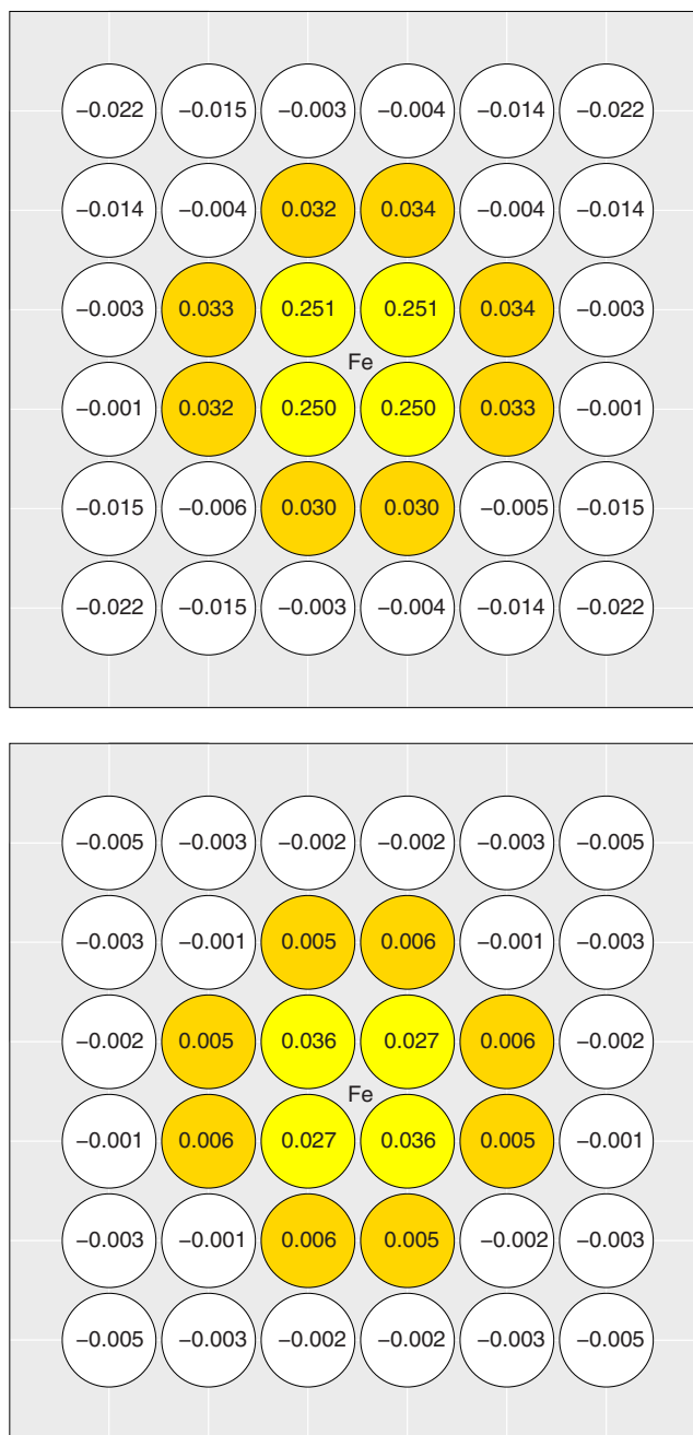
FIG. 7. (Color online) Magnetic spin (top) and orbital (bottom) moments on the Pd atoms in the surface layer induced by a single Fe adatom with an in-plane orientation of the magnetic moment (cf. text).
