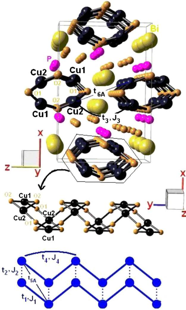
FIG. 1. (Color online) A schematic of the  $\text{BiCu}_2\text{PO}_6$  crystal structure is shown. It can be seen that two-leg ladders run along the crystallographic  $b$  direction. The two-leg ladder is separately shown for clarity. Also shown are the various significant hopping parameters and exchange couplings between Cu atoms.
