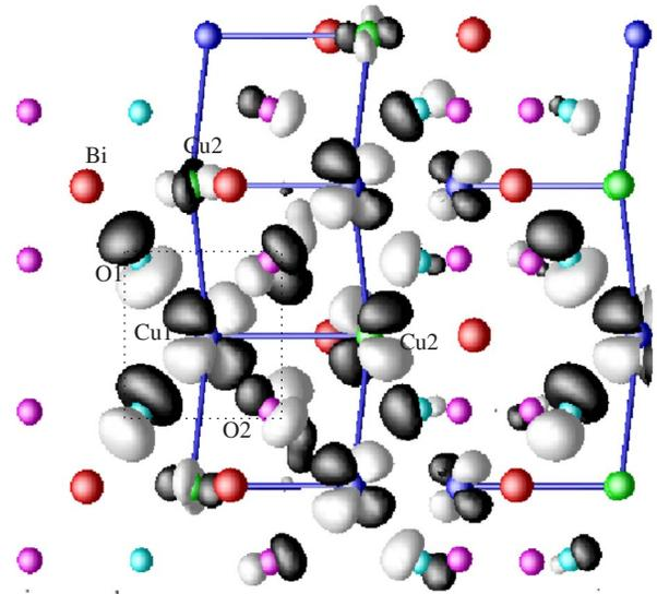
FIG. 5. (Color online) Effective Cu1  $d_{x^2-y^2}$  orbital with lobes of opposite signs colored as black and white. The  $d_{x^2-y^2}$  orbital is defined with the choice of the local coordinate system as discussed in the text (height of the isosurface =  $\pm 0.09$ ). The spheres represent the ions.
