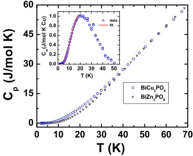
FIG. 3. (Color online) The measured heat capacity as a function of  $T$  for  $\text{BiCu}_2\text{PO}_6$  and  $\text{BiZn}_2\text{PO}_6$ . Inset: the magnetic specific heat of  $\text{BiCu}_2\text{PO}_6$  along with a fit (see text).
