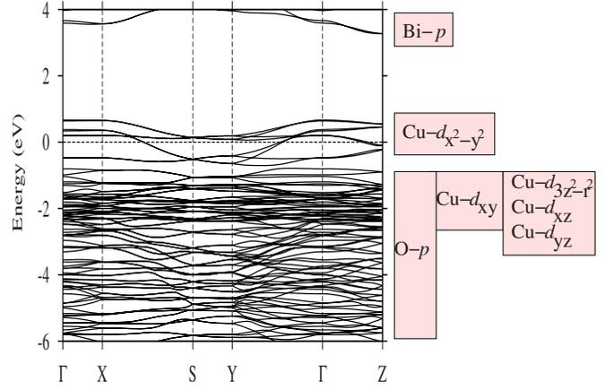
FIG. 4. (Color online) LDA band dispersion of  $\text{BiCu}_2\text{PO}_6$  along various symmetry directions.
