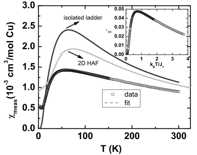
FIG. 2. Magnetic susceptibility ( $\chi_{\text{meas}}=M/H$ ) vs temperature  $T$  for  $\text{BiCu}_2\text{PO}_6$  in an applied field of 5 kG. The open circles represent the raw data and the dashed line is a fit (see text). Also shown are simulated curves for the isolated ladder (dark gray line) and for the 2D HAF (gray line). The inset shows the dependence of  $\chi^*$  on  $k_B T/J_1$  (see text).
