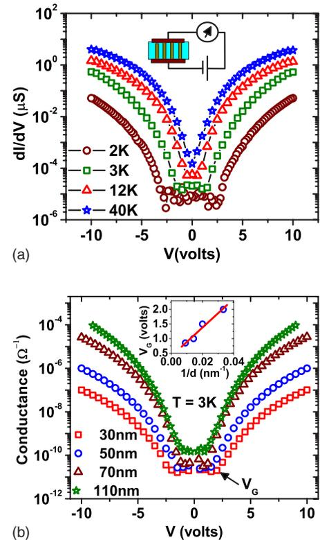
FIG. 1. (Color online) (a) Differential conductance ( $dI/dV$ ) is plotted as a function of bias voltage ( $V$ ) for a 30 nm diameter nanowire at various temperatures. Schematic diagram of the two-probe measurement configuration is shown in the inset. (b) Conductance vs voltage plot for four different diameter nanowires at  $T=3$  K. A gap voltage ( $V_G$ ) for 30 nm diameter nanowire has been indicated by an arrow.  $V_G$  has been plotted as a function of inverse diameter ( $d$ ) in the inset.
