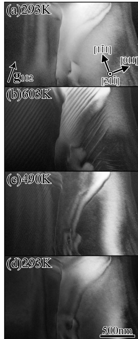
FIG. 12. Series of dark field images indicating the domain-structure change in the F_M side of the MPB. These images were taken at (a) 293 K before heating, and at (b) 603 K, (c) 490 K, and (d) 293 K on subsequent cooling, using the 102 reflection in the [21\bar{1}] electron incidence. When the temperature was raised above about 490 K, the new banded domain structure appeared in the interior of each domain in domain II.
