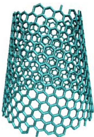
FIG. 3. (Color online) Schematic illustration of CNCs with R_t = 10 \text{ \AA} , R_b = 15 \text{ \AA} , and H = 30 \text{ \AA} .
