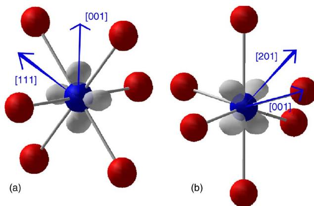
FIG. 12. (Color online) Orientation of  $d$  orbitals in (a) rutile and (b) anatase. The orbitals are obtained from charge-density difference analysis of the structures with and without an extra electron.
