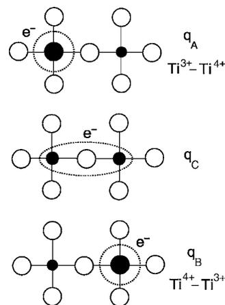
FIG. 1. Schematic diagram of polaron  $e^-$  transfer. In the initial state  $\Psi_A$  with structure  $q_A$ , the electron is localized on the left Ti ion, while in the final state  $\Psi_B$  with structure  $q_B$ , the electron is localized on the right Ti ion. At the transition state  $\Psi_C$  with structure  $q_C$  (a thermal transfer regime), the electron is shared between the two Ti ions.
