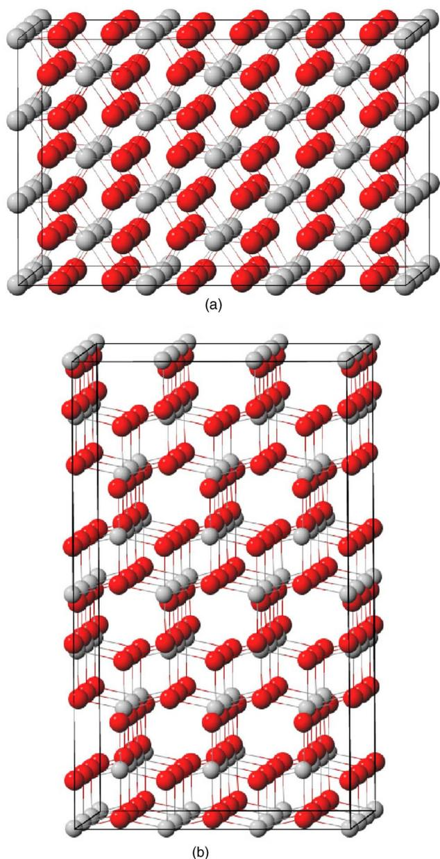
FIG. 3. (Color online) Bulk structures of  $\text{TiO}_2$  relevant to this study. (a)  $3 \times 3 \times 3$  rutile supercell. (b)  $3 \times 3 \times 2$  anatase supercell. Ti atoms are depicted as gray spheres, while O atoms red spheres.
