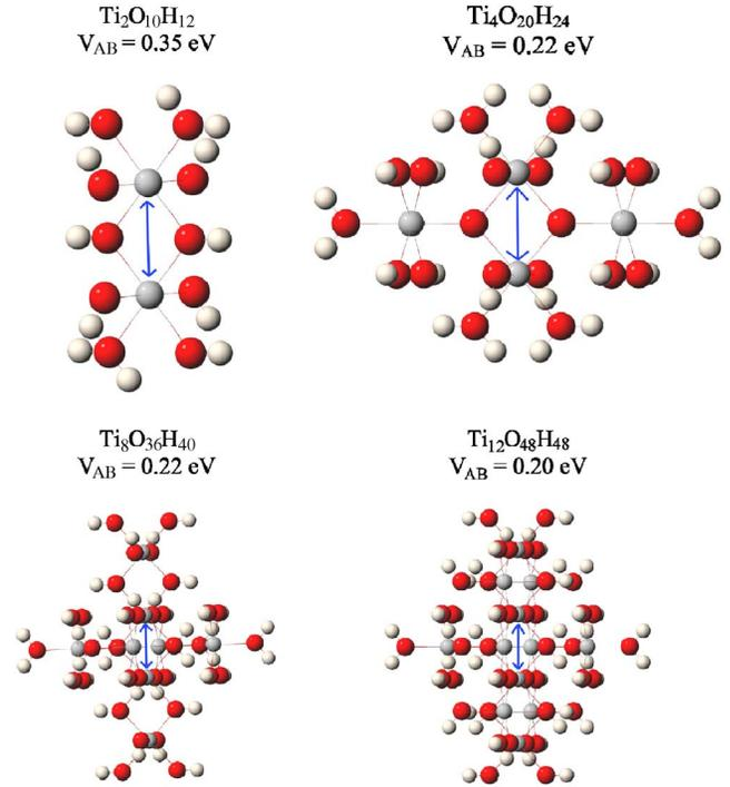
FIG. 10. (Color online) Clusters for  $V_{AB}$  calculations along [001] in rutile.
