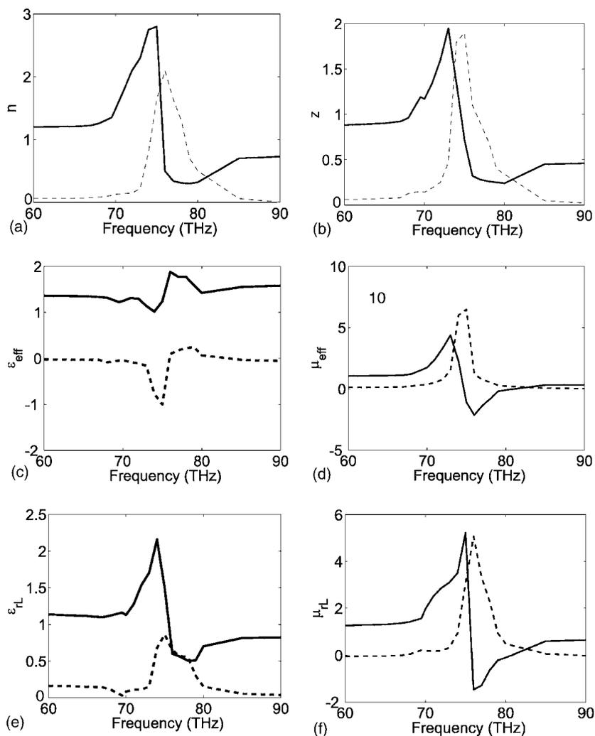
FIG. 5. (a) Refraction index extracted in Ref. 13 from  $R$  and  $T$  coefficients of a slab comprising the lattice of silver SRRs with period  $a=600$  nm. (b) Normalized Bloch impedance extracted in Ref. 13 (c) Nonlocal permittivity extracted for this lattice. (d) Nonlocal permeability. (e) Relative local permittivity. (f) Relative local permeability.
