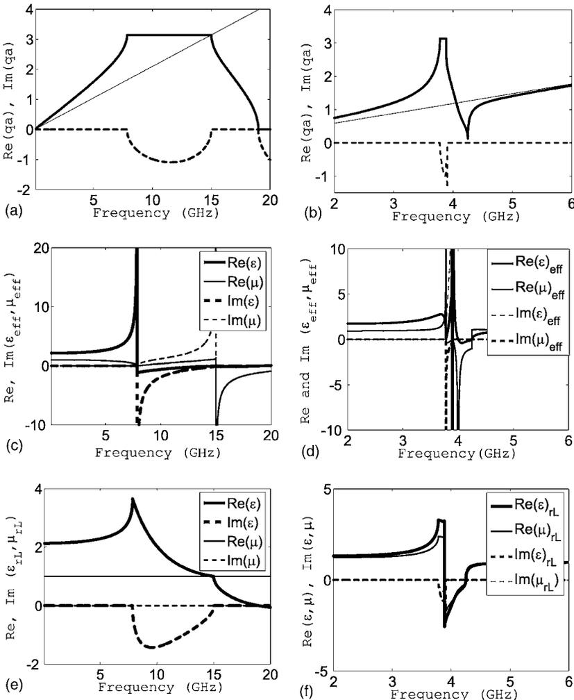
FIG. 4. (a) Dispersion in a lattice of nonresonant dipoles. (b) Dispersion in a lattice of resonant p-m particles (pairs of  $\Omega$  particles). (c) Nonlocal MP for the lattice of nonresonant dipoles. (d) Nonlocal MP for p-m particles. (e) Local MP for nonresonant dipoles (locality is satisfied up to the spatial resonance of the lattice at 7.5 GHz). (f) Local MP for p-m particles (pairs of  $\Omega$  particles).
