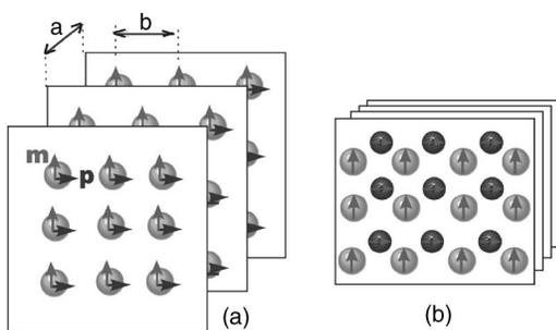
FIG. 1. Presentation of a p-m lattice as a set of dipole crystal planes. (a) Every particle has both electric and magnetic moments. (b) Electric and magnetic particles are different.
