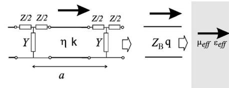
FIG. 2. Presentation of a lattice with electric and magnetic inclusions (p-m lattice) as (1) periodically loaded transmission line, (2) homogenized transmission line with Bloch impedance  $Z_B$  and wave number  $q$  ( $k$  and  $\eta$  are unloaded wave number and characteristic impedance, respectively), and (3) effective magnetodielectric medium with nonlocal MP  $\epsilon_{\text{eff}}$  and  $\mu_{\text{eff}}$ .
