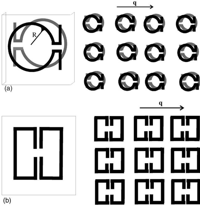
FIG. 3. (a) Lattice of pairs of  $\Omega$  particles operating at microwaves. (b) Lattice of SRRs operating at infrared suggested by O'Brien and Pendry (Ref. 11).
