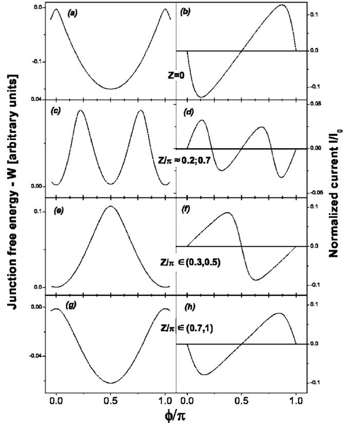
FIG. 4. Free energies and current-phase relations of junctions at low temperature  $T = 0.05T_c$  corresponding to stable states in Fig. 2 (see text). Note the unusual shapes of the CPR: (d) close to deformed  $I(\phi) \sim \sin(4\phi)$  curve, (f) close to  $I(\phi) \sim \sin(2\phi)$ , and (h) close to  $I(\phi) \sim \sin(2\phi + \pi)$ .
