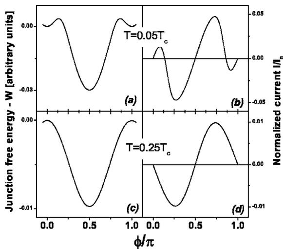
FIG. 5. Free energies and corresponding CPR for an example of coexistence of stable  $\pi/2$  and metastable  $0$  and  $\pi$  states,  $Z=0.1\pi$ , at low and at higher temperatures.
