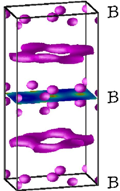
FIG. 2. (Color online) Isosurface of  $\text{Li}_2\text{B}_2$  charge density corresponding to the  $\zeta$  state near the Fermi level, halfway between the  $\Gamma$  and A points. The top, center, and bottom planes in the figure contain honeycomb sheets of B. The charge density in the center B plane is shown. Two Li layers lie between each pair of B sheets. The  $\zeta$  states are primarily concentrated in the interlayer region, but have some B  $p_z$  character as well.
