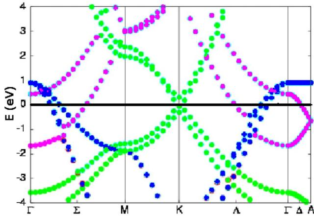
FIG. 1. (Color online)  $\text{Li}_2\text{B}_2$  band structure near the Fermi level ( $E_F=0$ ). The  $\sigma$ ,  $\pi$ , and  $\zeta$  bands are plotted with blue (black), green (dark gray), and magenta (light gray) symbols, respectively. Note that in the directions plotted, the  $\pi$  bands (green or dark gray) cross the Fermi level only at the K point.
