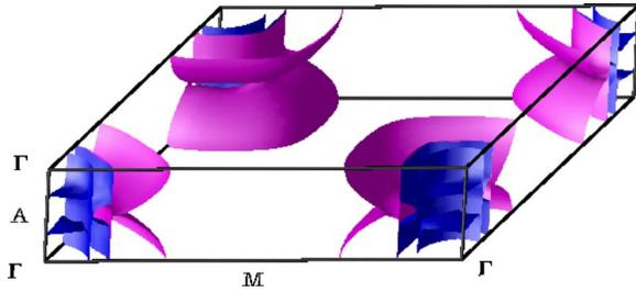
FIG. 3. (Color online) Fermi surface of  $\text{Li}_2\text{B}_2$ . The cylindrical sheets centered on the  $\Gamma$ -A line arise from the 2D  $\sigma$  bands, while the ellipsoids are due to free-electron-like  $\zeta$  bands.
