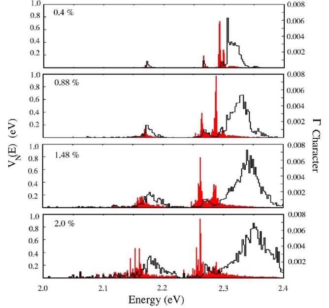
FIG. 4. (Color online) Black open histograms: calculated N-state energies weighted by the square of their interaction with the  $\Gamma$  CB minimum. Red (gray) filled histograms:  $G_\Gamma(E)$ , the projection of the N-state spectrum onto the unperturbed GaP  $\Gamma$  state.
