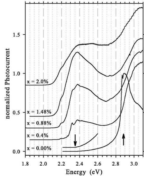
FIG. 2. Normalized and response-corrected PC spectra of the series of  $\text{GaN}_x\text{P}_{1-x}$  samples with  $x$  up to 2.0% (20 K). Arrows indicate the GaP indirect and direct band gaps.
