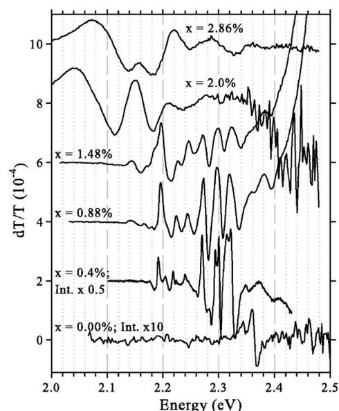
FIG. 1. EA spectra of the series of  $\text{GaN}_x\text{P}_{1-x}$  samples (20 K).  $dT/T$  denotes the relative change in transmission.
