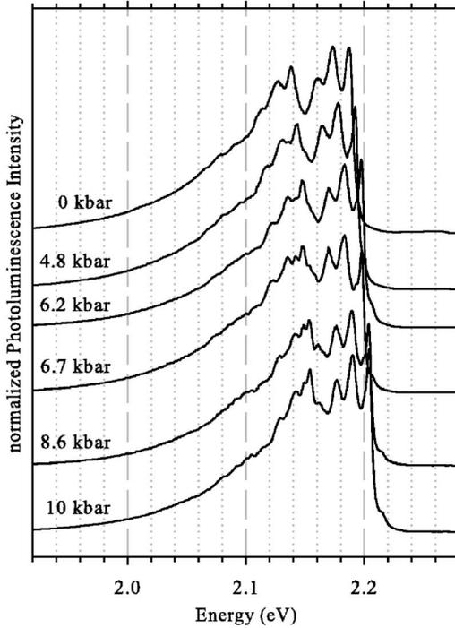
FIG. 3. Normalized PL spectra of a  $\text{GaN}_{0.003}\text{P}_{0.997}$  at different hydrostatic pressures (5 K, UV excitation).
